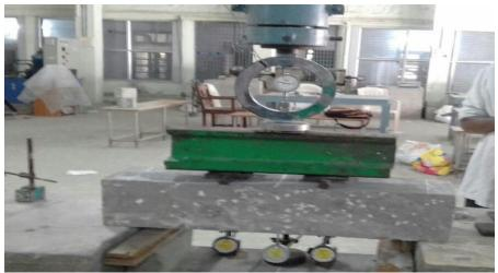
Figure 2: Flexural Testing Machine
