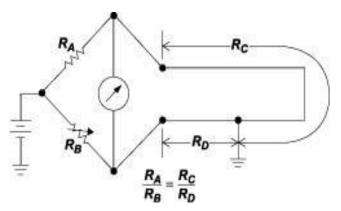
Figure 1 :Murray loop test
