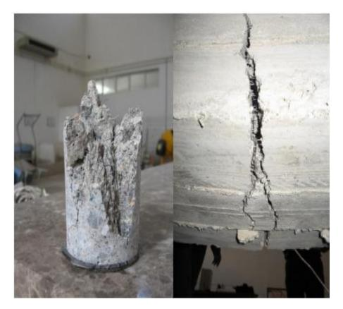
Fig4.1. Fiber added material for bridging cracks.
