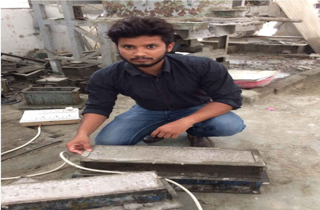
Figure: 4 casting specimen for Flexural Strength test Flexural strength for different proportions of cnsl resin for 28 days is as follows:
