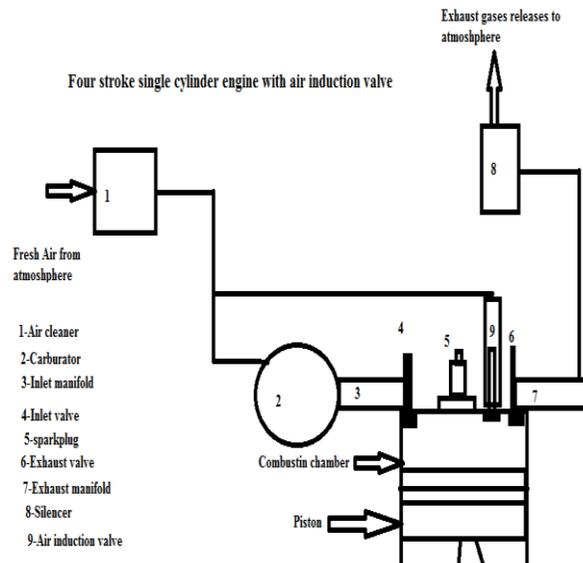
Working of A ir-induction valve engine is similar to conventional single cylinder four stroke engines.
