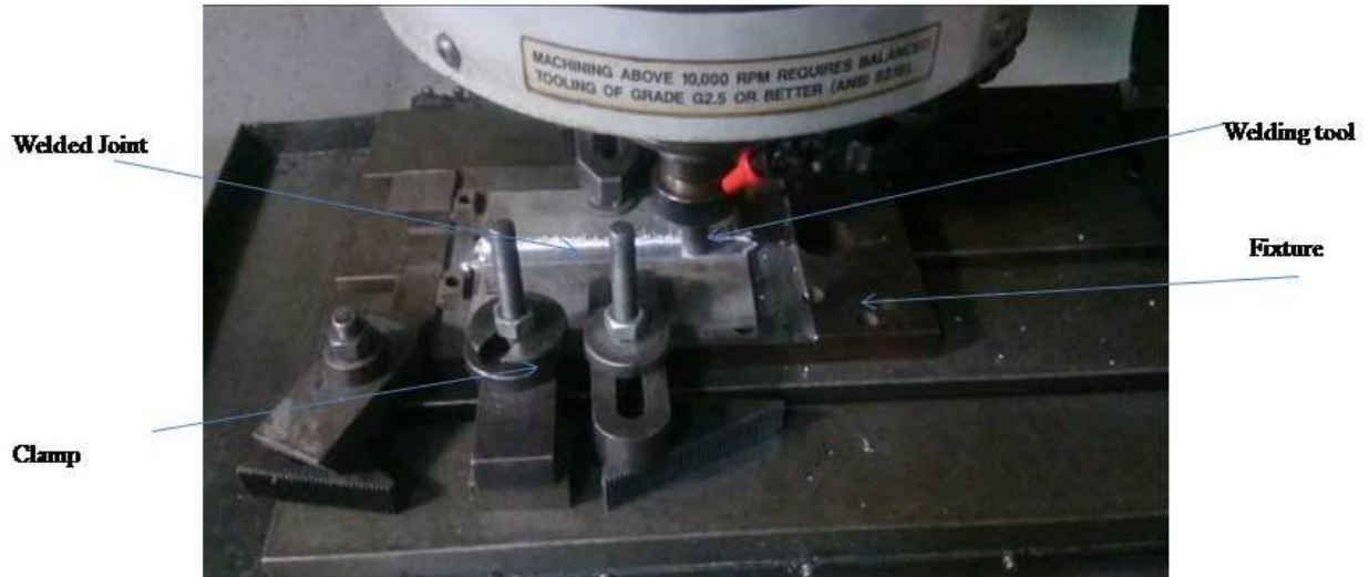
Figure 2. Work piece set up during FSW
