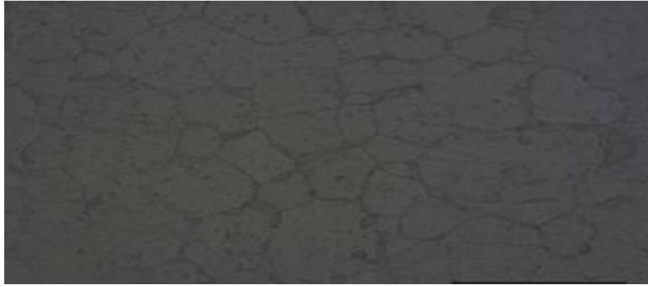
Figure 9. Microstructure of Aluminium 6106
