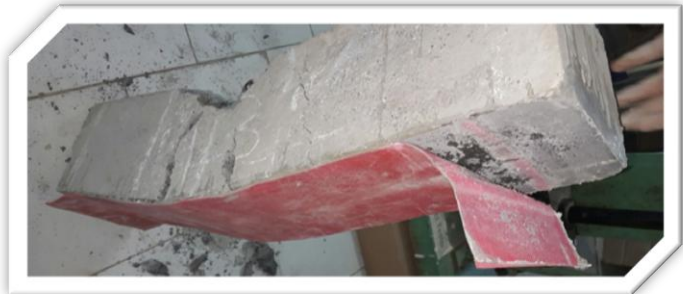
Figure 4: Crushing of concrete in compression and debonding of polypropylene fabric of triple layer
