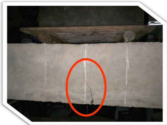
Figure 3: Flexural failure of reference beam
