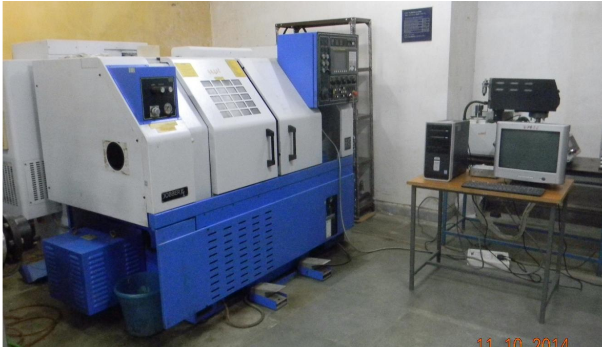
Figure 2. Experimental set up of CNC lathe
