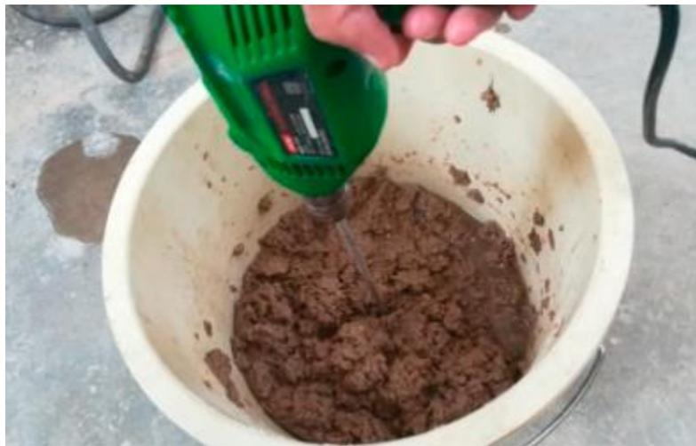
Figure 3: Sand and Zeolite mixing through mechanical vibrator
