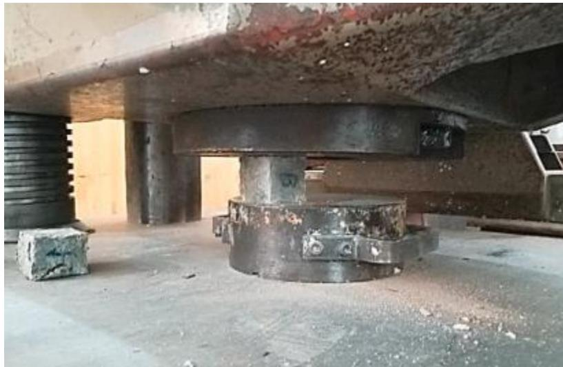
Figure 5: Type B specimen during compression test
