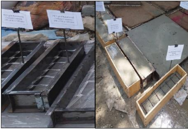
Figure 6. (150 x 150 x 700)mm PCC, PET-CC, RCC beams Figure 7. Concrete slabs and molded beams after casting
