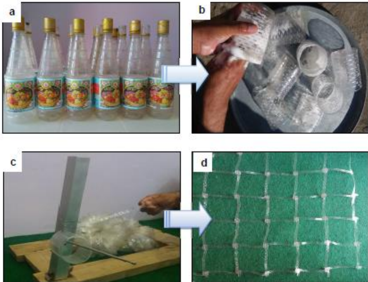
Figure 1. Fabrication of PET Grid: (a) Collection of PET beverages bottles; (b) Rinsing of cut imprinted bottles with detergent; (c) strips extraction; (d) fabrication of PET grid
