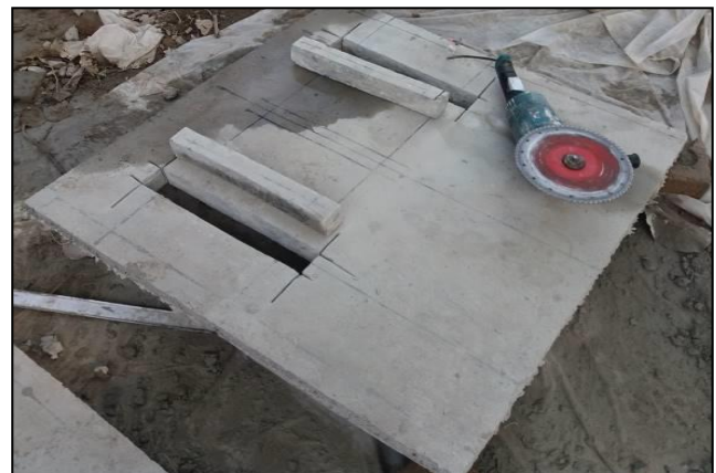
Figure 9. Sawing beams from slabs
