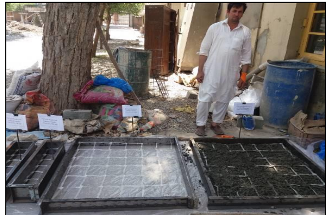
Figure 3. 1m x 1m x 100mm PET-grid reinforced cement concrete slab
