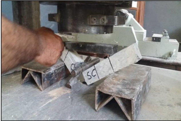
Figure 9. Sawed beams of CSC for flexure strength test after rupture
