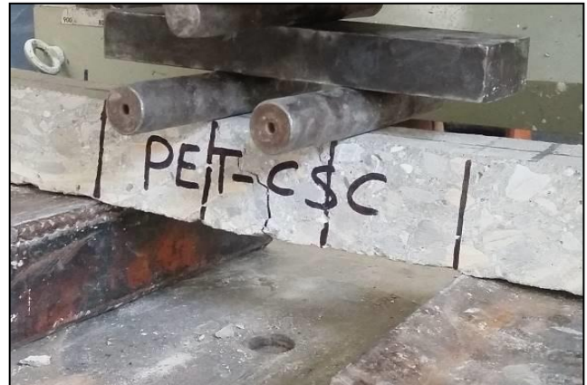
Figure 10. Sawed beams of PET-CSC for flexure strength test after rupture
