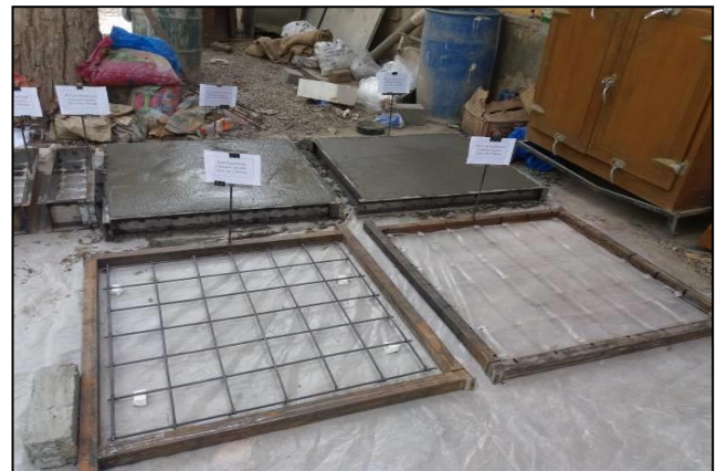
Figure 5. 1 m x 1 m x 50 mm PET-grid reinforced and steel reinforced concrete slab
