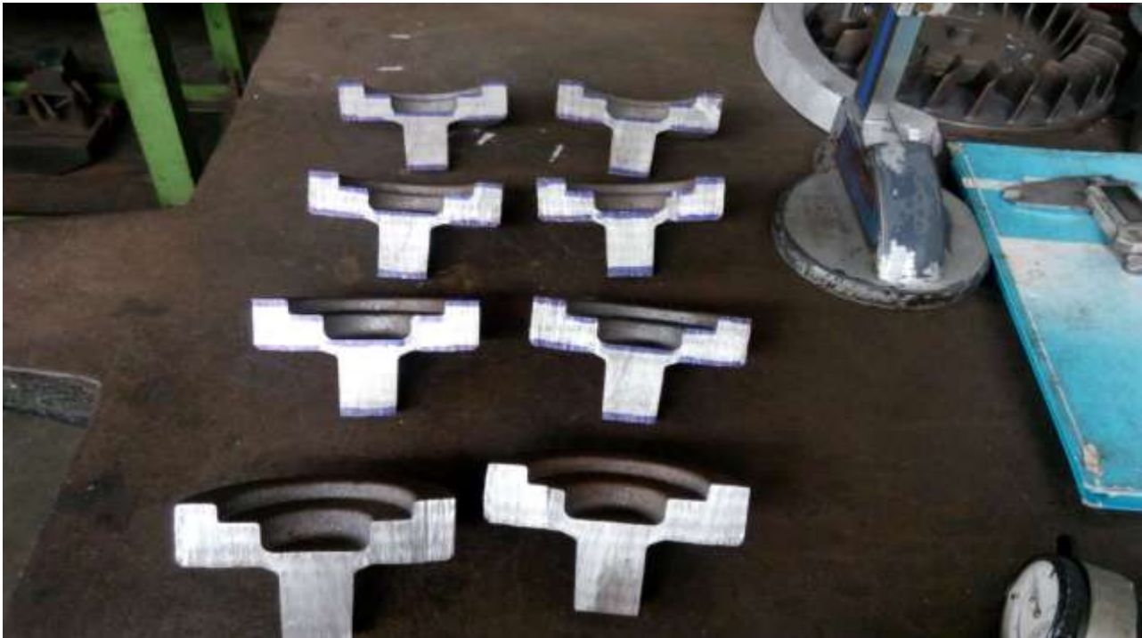
Figure 8. cross sections shows no internal porosity of component after implementation of iteration 3
