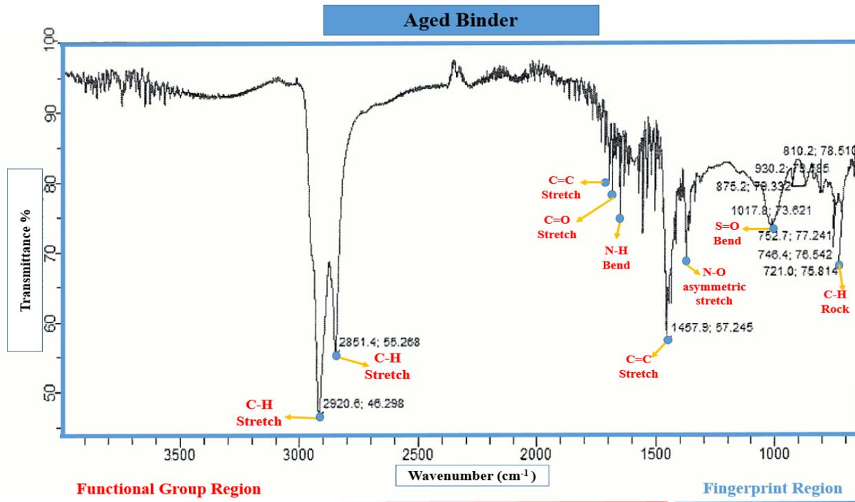
Figure 10. FTIR spectrograph of aged bitumen sample
