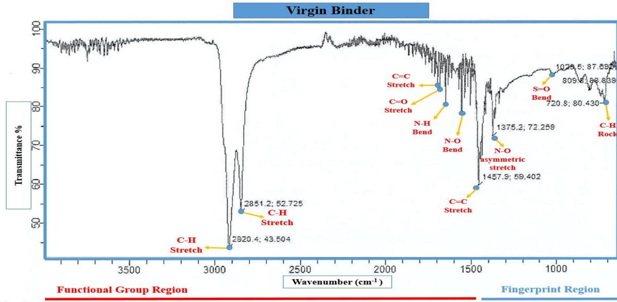
Figure 7. FTIR spectrograph of virgin bitumen sample
