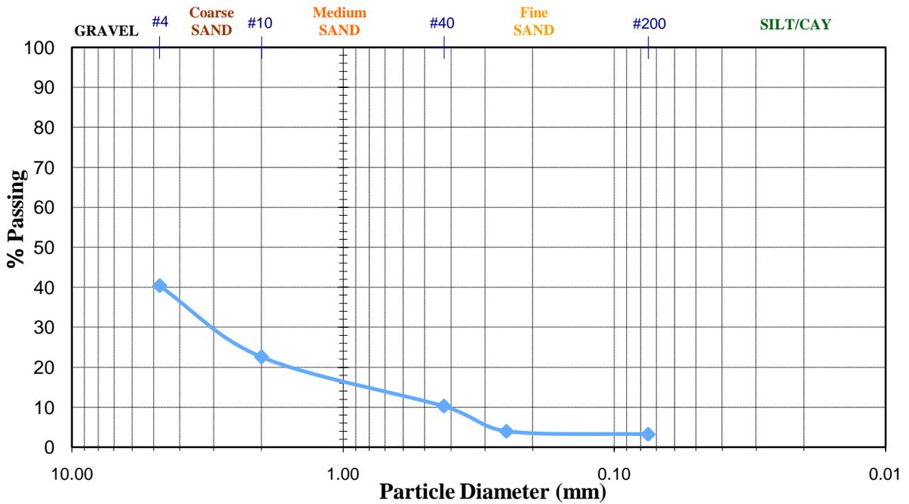
Figure 9. Grain size distribution in the asphalt base course
