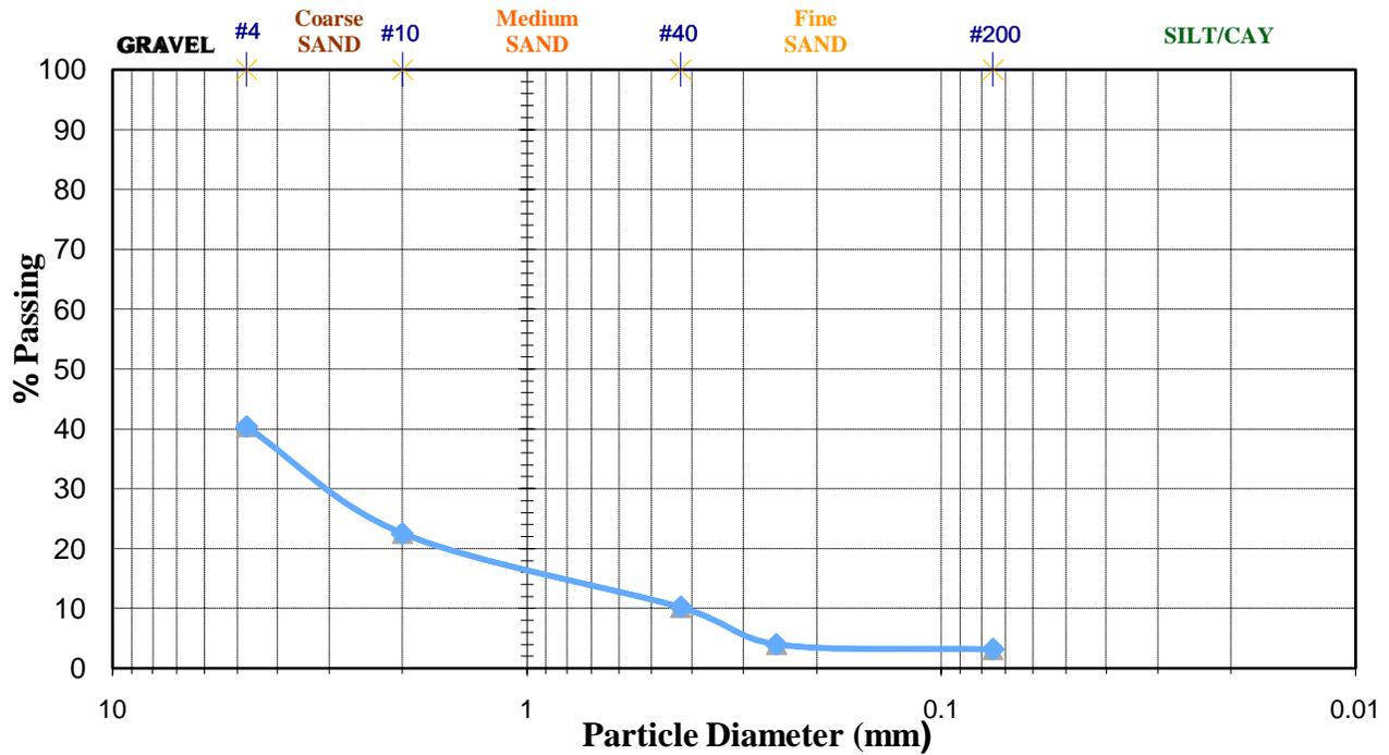
Figure 8. Grain size distribution in the asphalt wearing course
