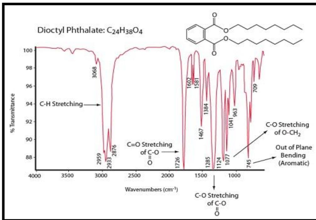
*Figure 1. Typical image of spectrograph made by an FTIR Spectrometer*
