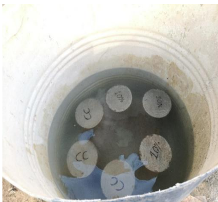
Figure 17. Curing of Cylinders
