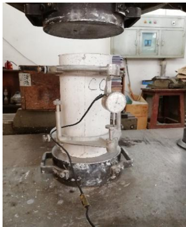
Figure 5. Cylinder Placed in UTM
