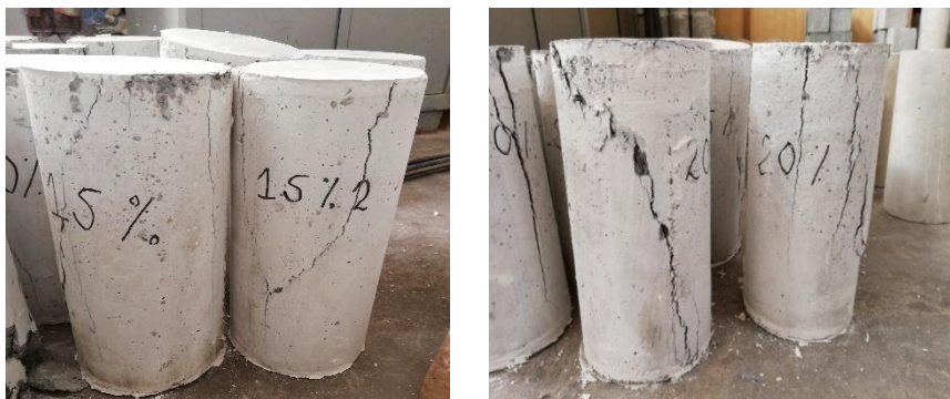
Figure 24. Cylinders Tested for Compressive Strength
