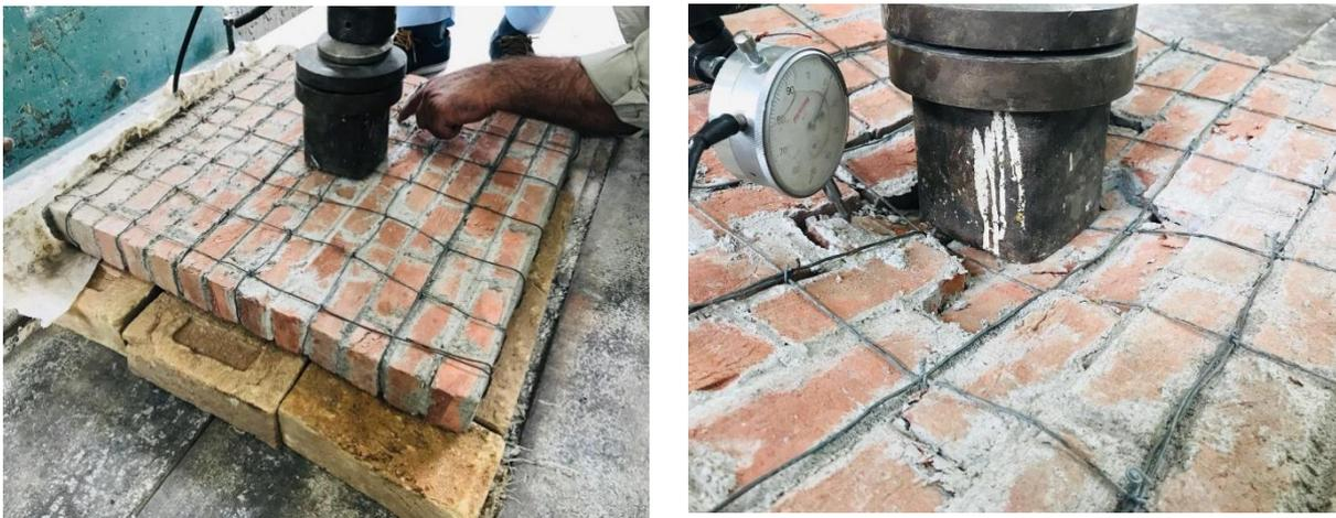
Figure 5 shows test setup of out-of-plane masonry prisms with containment
