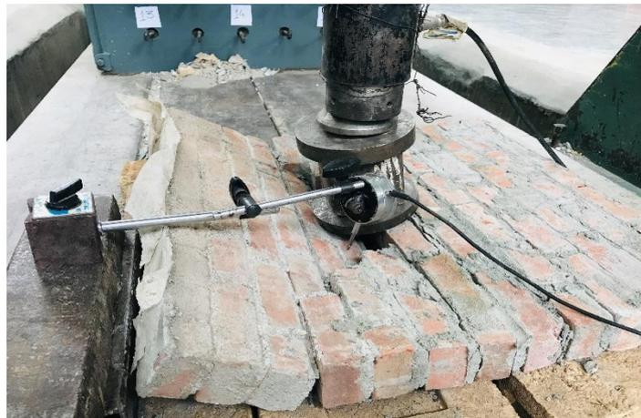
Figure 6 shows test setup of out-of-plane without containment
