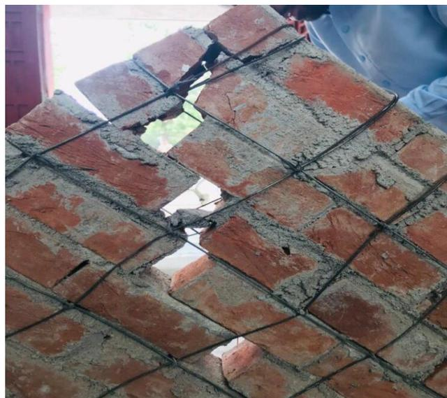
**Figure 4.** Diagonal crack in masonry prism
