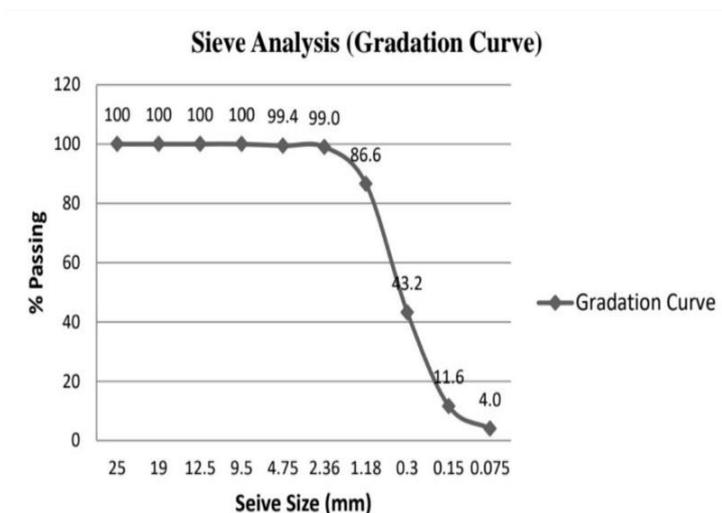
**Figure 1** shows sieve analysis of sand
