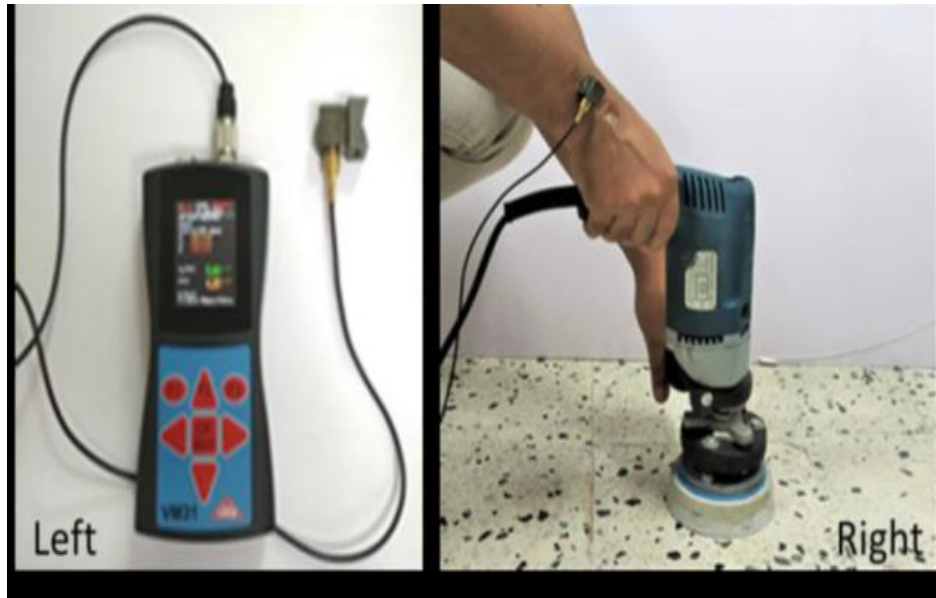
Fig. 2. Hand-arm vibration meter connected with the tri-axial accelerometer (left-image) and tri-axial accelerometer on the wrist of the operator during use of a polishing machine (right-image)
