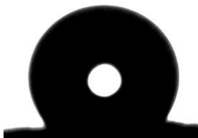
Fig.4.d. Contact of water over a thin film of PVC containing metallic stearate coated on Al film. CA= 133.6^\circ
