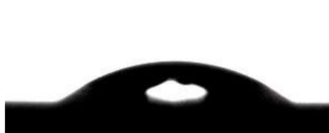
Fig.4.a. Contact of water with glass substrate. CA= 27.4^\circ
