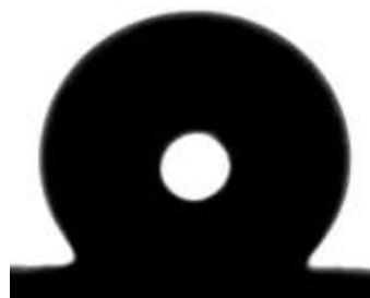
Fig.4.e. Contact of water over a thin film of PVC containing metallic stearate & nano copper oxide on Al film. CA= 137.5^\circ
