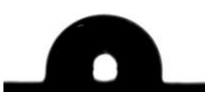
Fig.4.b. Contact of water with nano aluminium film. CA= 96.4^\circ
