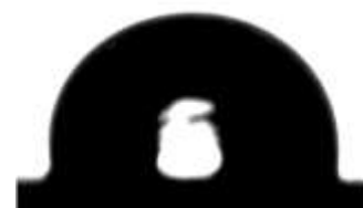
Fig.4.c. Contact of water over a thin film of PVC coated on Al film. CA= 101.6^\circ
