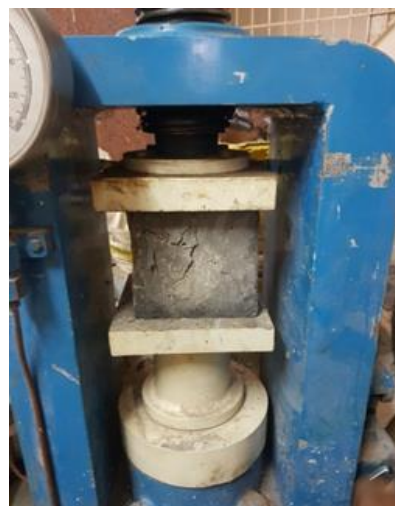
Fig: 2 Testing of mortar cubes in compression machine
