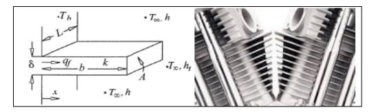
Figure 3.3: Structure of fins
