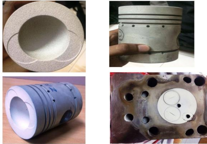
Figure 2 Thermal Barrier Coating on Piston Crown, Cylinder Head and Valves
