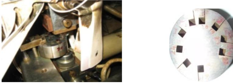
Fig. 2.1 Specimen after Machining: Size - Dia. 60mm and Thickness 40 mm
