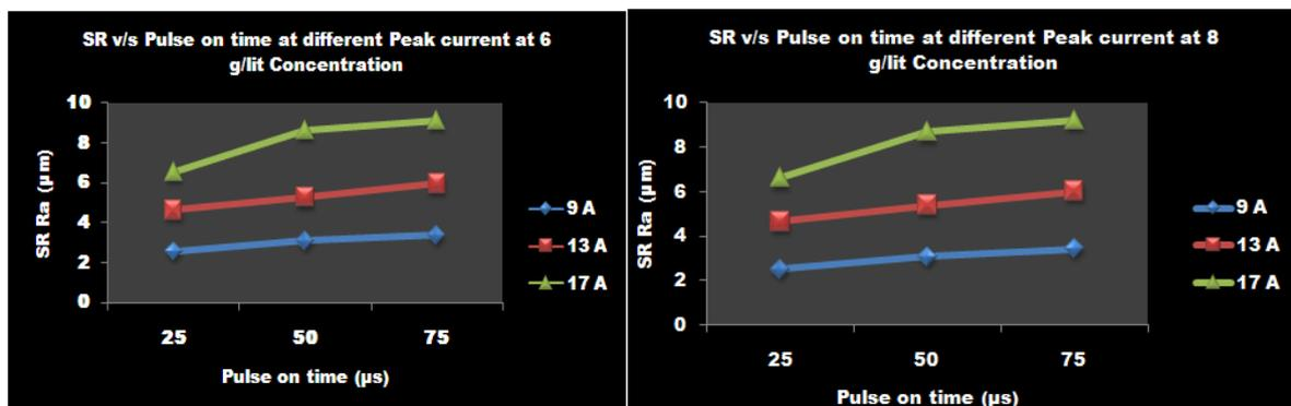
Figure 1.7: SR v/s Pulse on time at different Peak current at 6 & 8 g/lit Concentration
