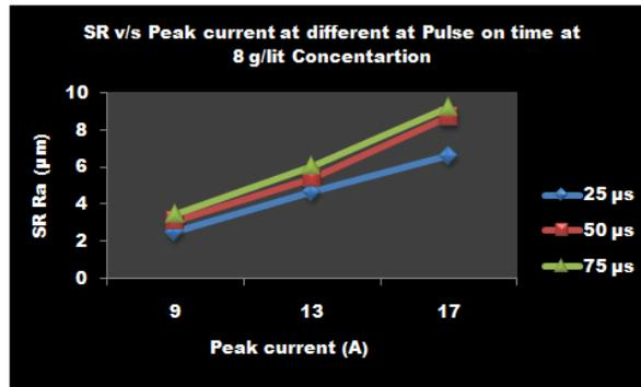
Figure 1.4: SR v/s Peak current at different Pulse on time at 4, 6 & 8 g/lit concentration
