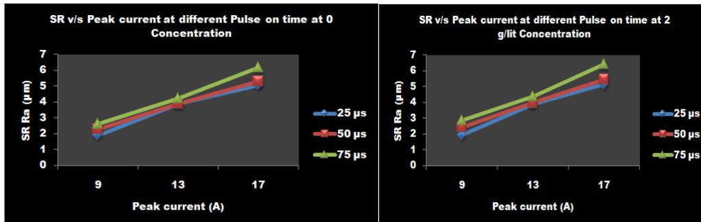
Figure 1.3: SR v/s Peak current at different Pulse on time at zero & 2 g/lit concentration
