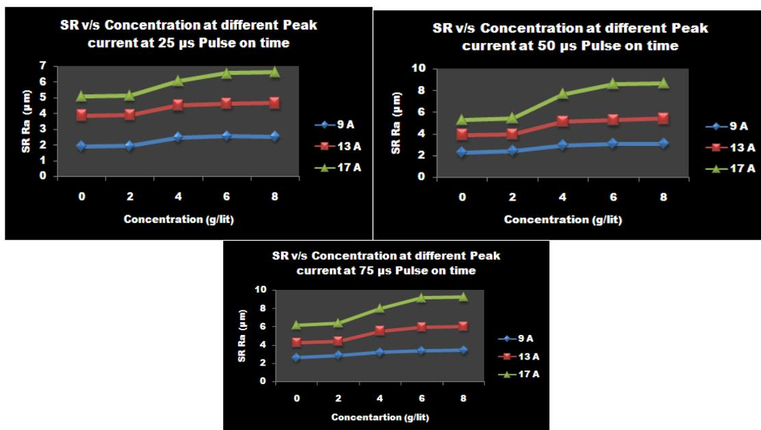
Figure 1.5: SR v/s Concentration at different Peak current at different Pulse on time
