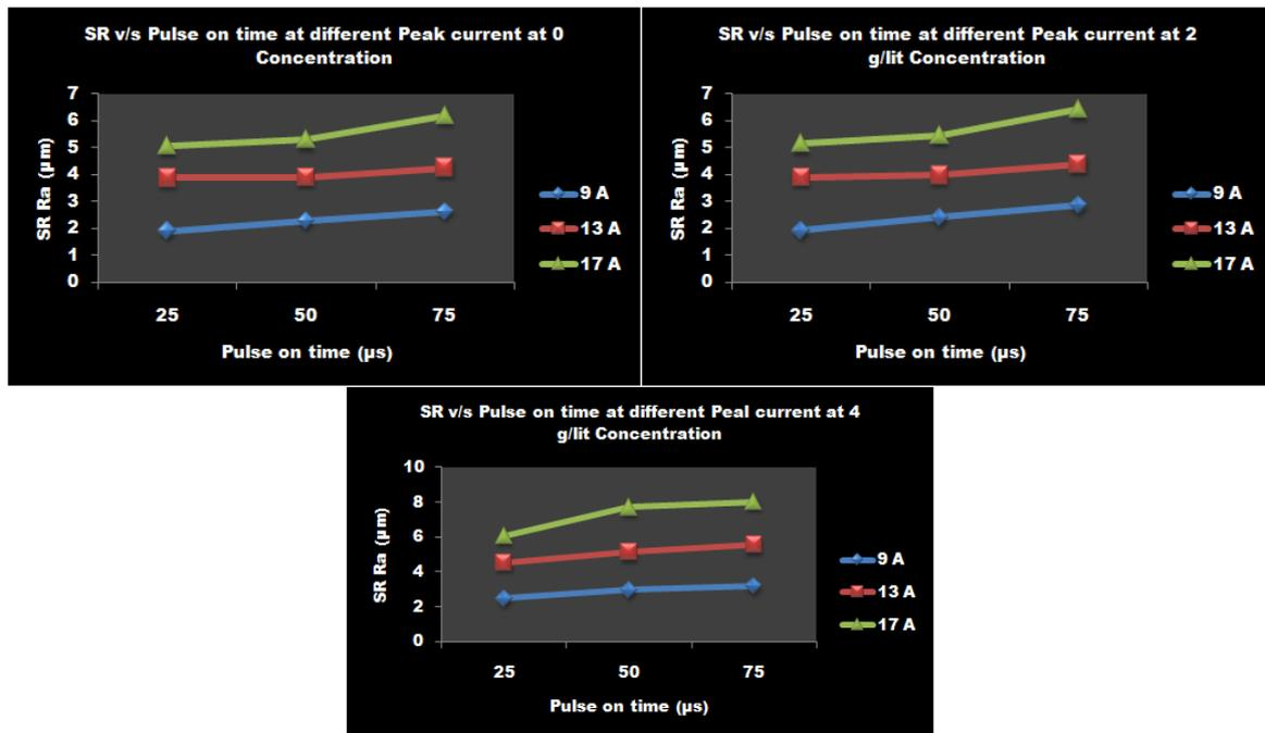
Figure 1.6: SR v/s Pulse on time at different Peak current at zero, 2 g/lit & 4 g/lit Concentration
