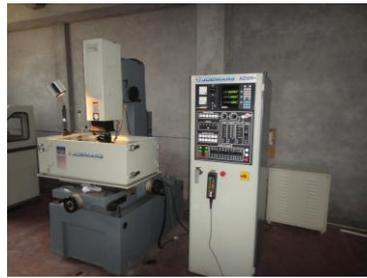
**Figure .1.2 Electro Discharge Machine used for performing experiments**
