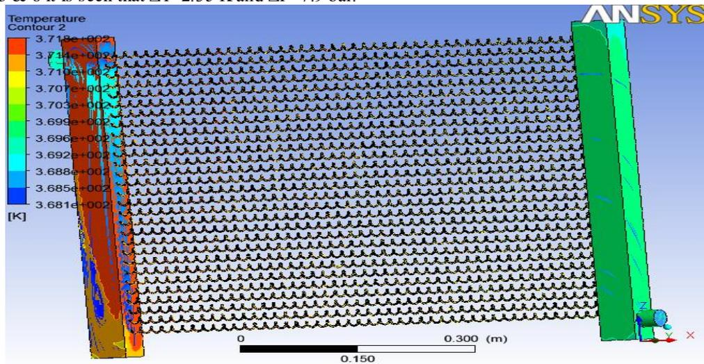
Figure 7: Temperature diagram of helical tubes used in Radiator. (Propylene Glycol)
