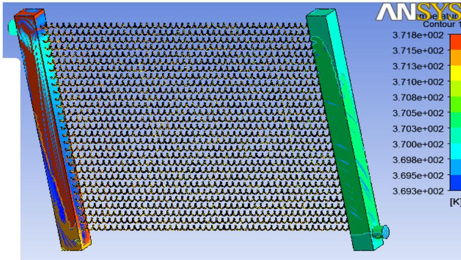
Figure 17: Temperature diagram of helical tubes used in Radiator. (Propylene Glycol)
