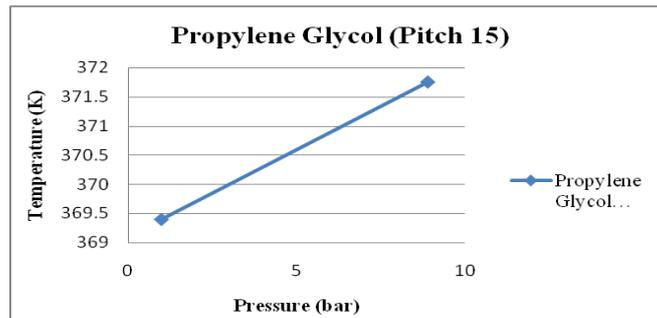
Figure 6: Inlet & Outlet Temperature VS Inlet & Outlet Pressure of Helical Tube (Propylene Glycol)
