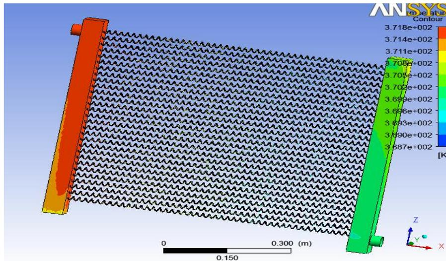
Figure 20: Temperature diagram of helical tubes used in Radiator. (Methanol)
