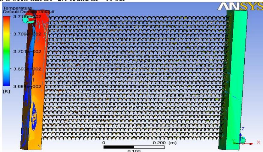
Figure 4: Temperature diagram of helical tubes used in Radiator. (Ethylene Glycol)
