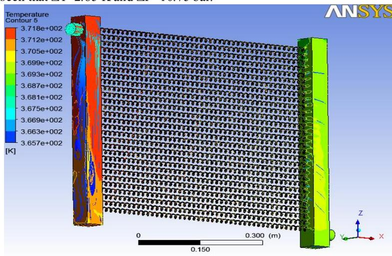
Figure 10: Temperature diagram of helical tubes used in Radiator. (Methanol)
