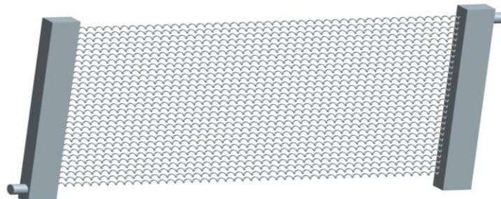
**Figure 1: Helical tube radiator in Pro-E**
