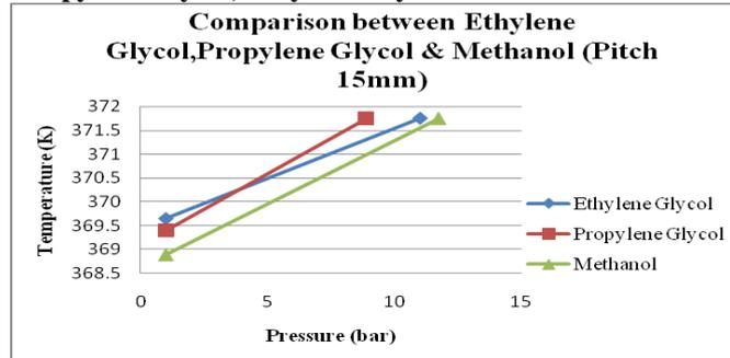
Figure 11: Comparison of Propylene, Ethylene Glycol & Methanol. (Helical Tube-15mm pitch)
