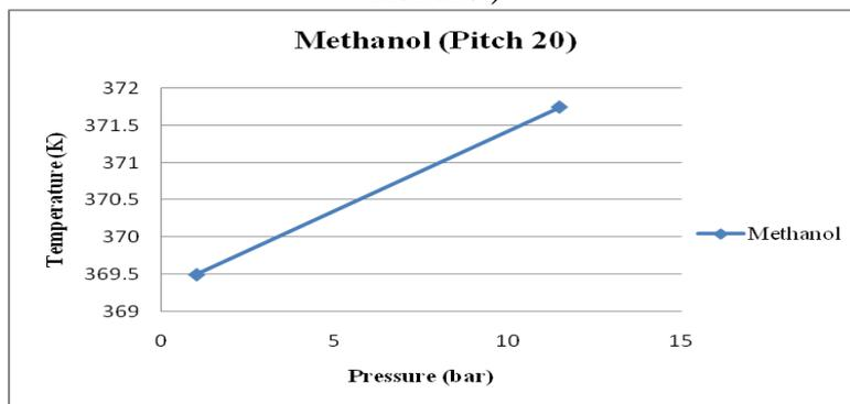
Figure 19: Inlet & Outlet Temperature VS Inlet & Outlet Pressure of Helical Tube (Methanol)
