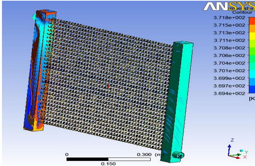
Figure 14: Temperature diagram of helical tubes used in Radiator. (Ethylene Glycol)
