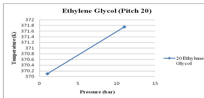
Figure 13: Inlet & Outlet Temperature VS Inlet & Outlet Pressure of Helical Tube (Ethylene Glycol)
