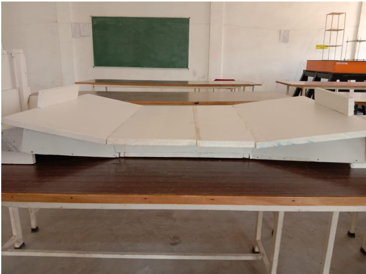
Completed model of canal syphon
