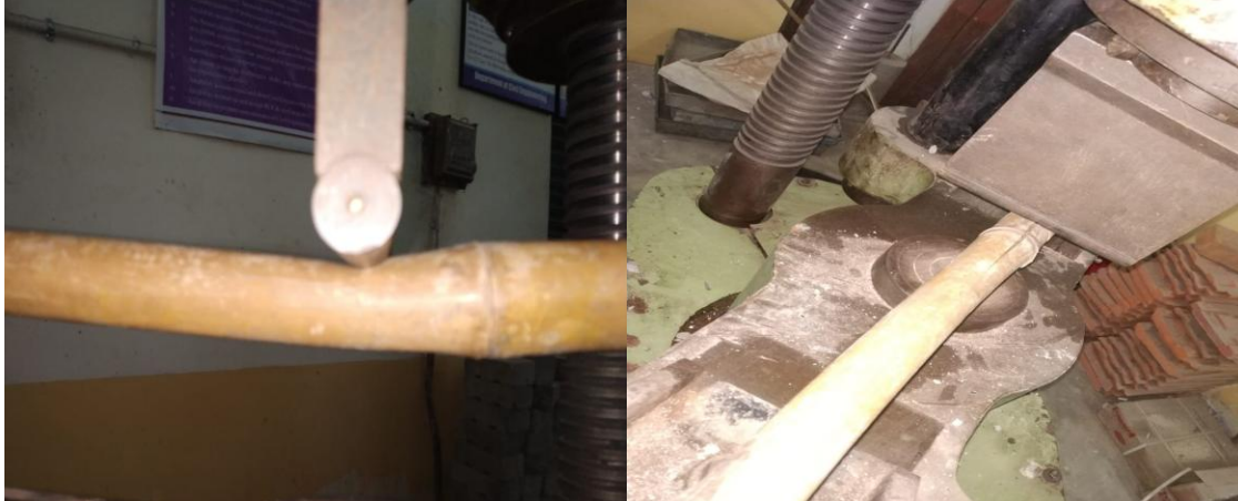
Fig. (a): Loading applied to Bamboo Fig. (b): Flexural strength on Bamboo
