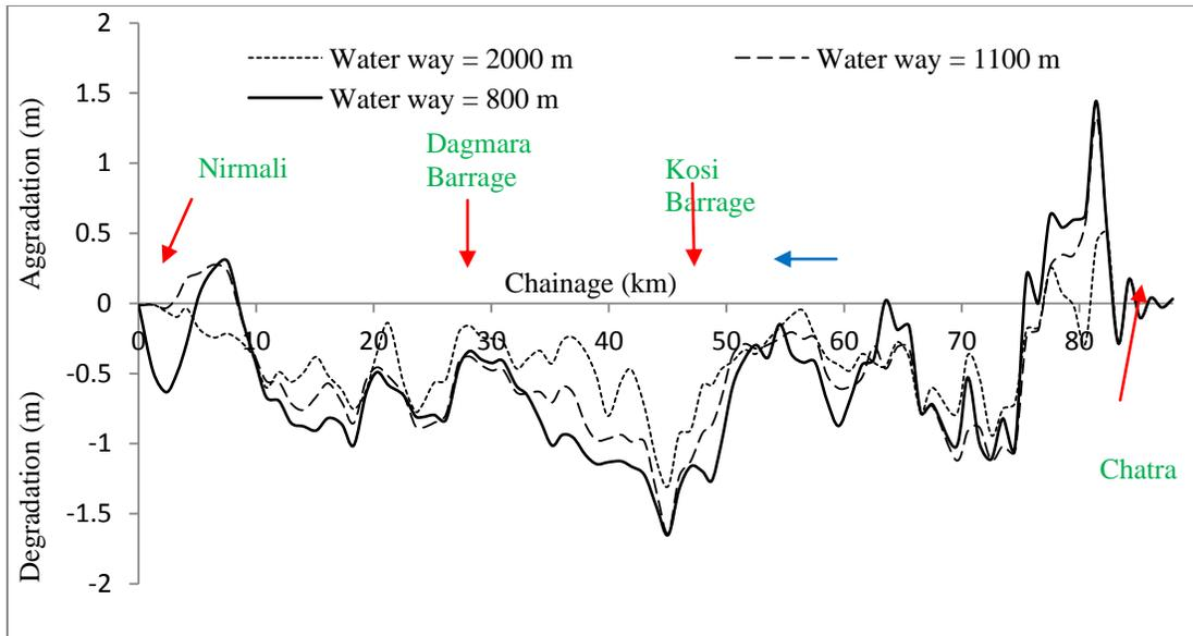
**Figure 2** Morphological changes of bed level with respect to river bed level of year 2002 (Burele el al., 2014)
