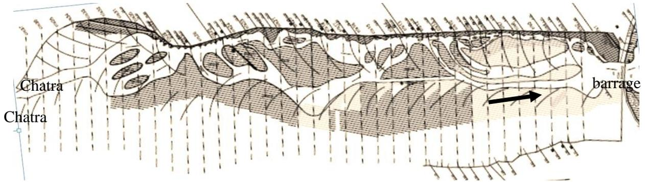
**Figure 15** Plan showing layout of embankment and showing position of hockey stick shape groynes for a reach from Chatra to Kosi barrage (Waterway = 1,100 m,)
