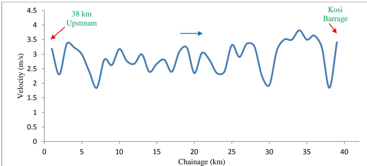
**Figure 19** Velocity along the river for  $Q = 15,586 \text{ m}^3/\text{s}$
