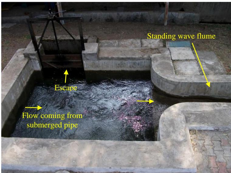
Figure 7 Shows standing wave flume from where the measured discharge is taken in to model
