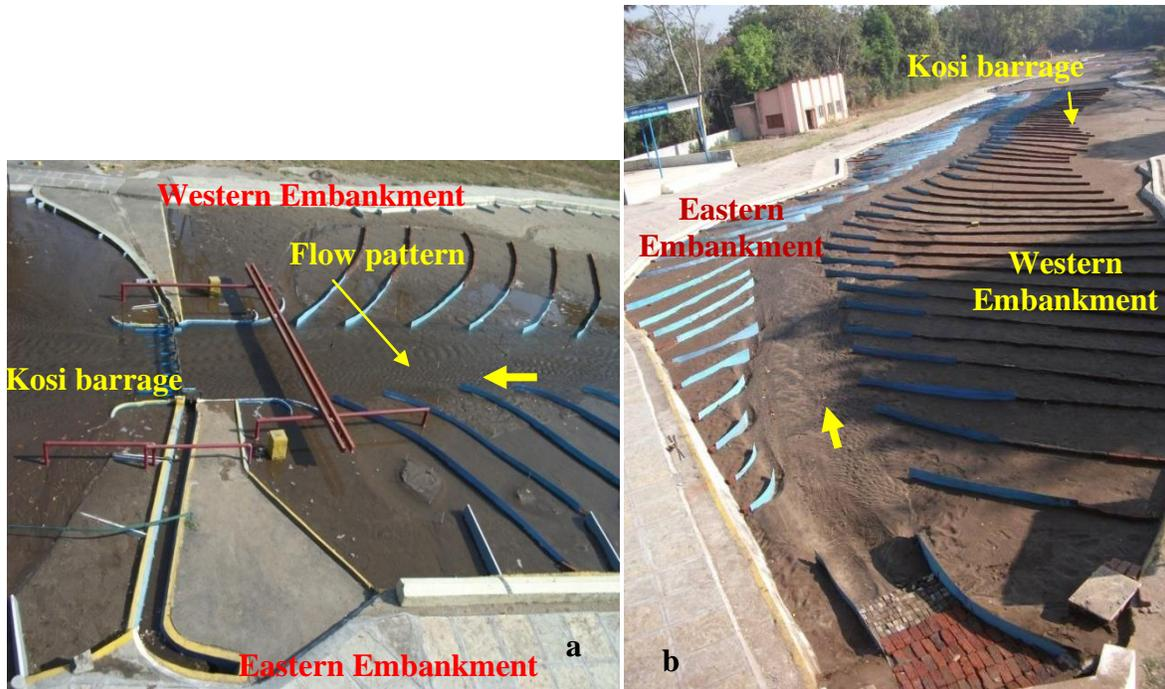
**Figure 18**a) Side view of model with a discharge of  $15586 \text{ m}^3/\text{s}$  at Barrage b) Upstream view of model showing bed formation after a discharge of  $15586 \text{ m}^3/\text{s}$
