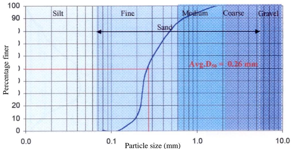
**Figure 11** Grain size distribution curve of bed material used in the model
