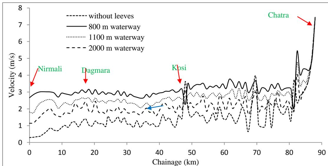
**Figure 3** Velocity distributions longitudinally for various channelization width (Burele el al., 2014)
