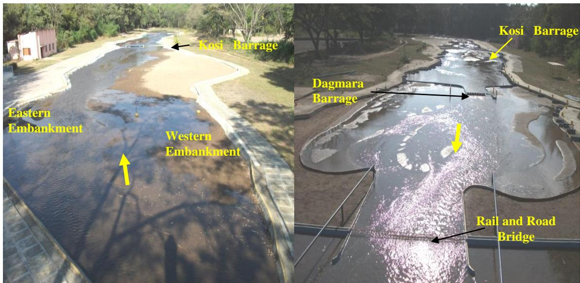
**Figure 13 a)** upstream View **b)** A downstream view of the model ( $Q = 15,586 \text{ m}^3/\text{s}$ )
