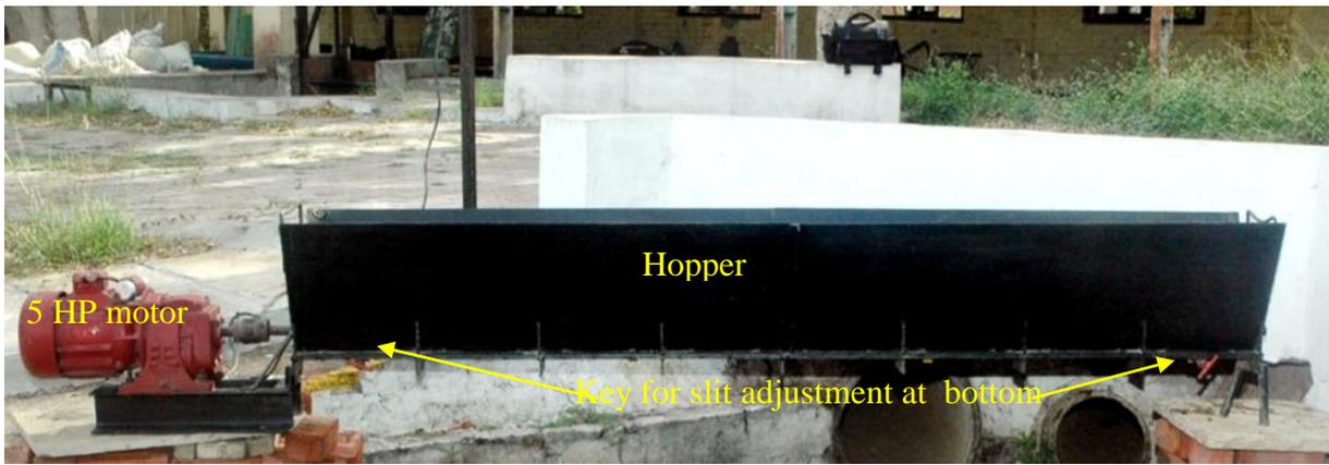
Figure 6 Silt injector(Front view)
