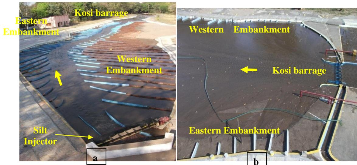
**Figure 17** a) Upstream view of model with a discharge of  $15586 \text{ m}^3/\text{s}$  for a reach from Chatra to Barrage b) Side view of model near barrage showing flow pattern for discharge of  $15586 \text{ m}^3/\text{s}$
