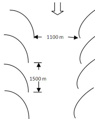
**Figure 16** a) Channel configuration showing position of hockey stick shape groynes from Chatra to Barrage b) Detail of hockey stick shape groynes provided in the model
