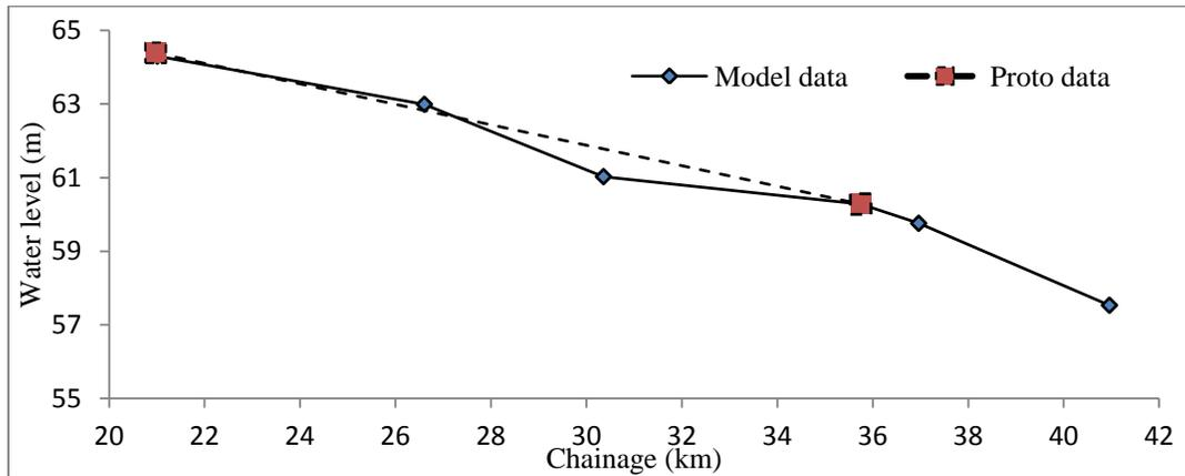
**Figure 12** Comparison between observed and recorded water level for  $Q = 10,960 \text{ m}^3/\text{s}$
