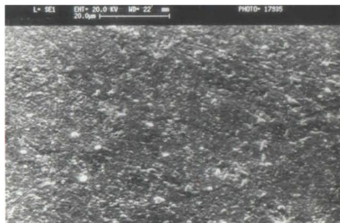
SEM Micrograph of composite with 10wt. % micron SiC
