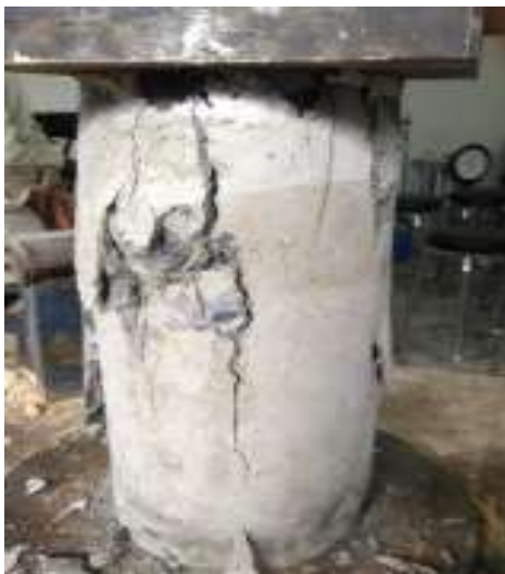
Figure 3: Compressive Strength Test
