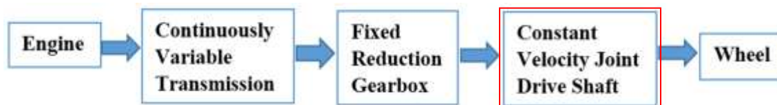
Figure 1. Typical power flow in transmission system
