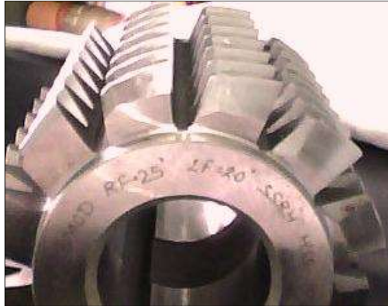
Fig. 15 Developed hob with 25^{\circ} - 20^{\circ} pressure angle
