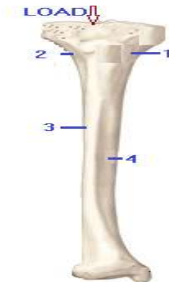
Fig.2 Bonding of strain Gauges at Various Positions
