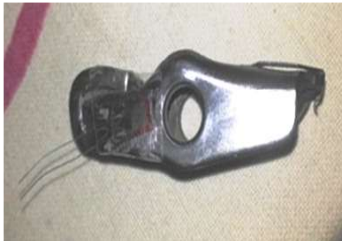
Fig.7.Strain Gauge Mounted on rocker arm
