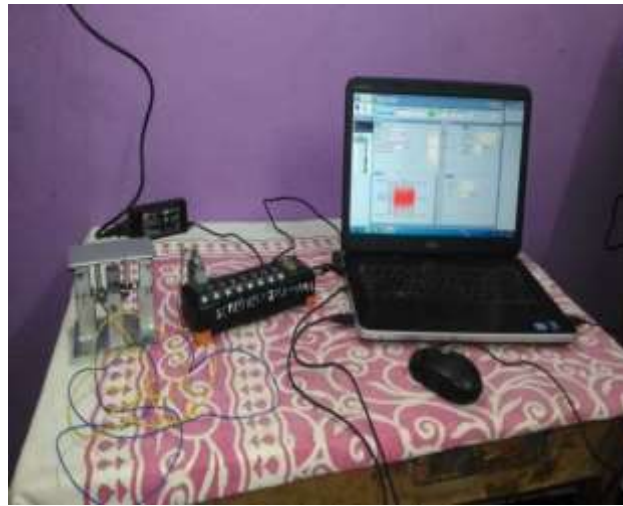
Fig.8.Experimental Setup of Strain Gauge
