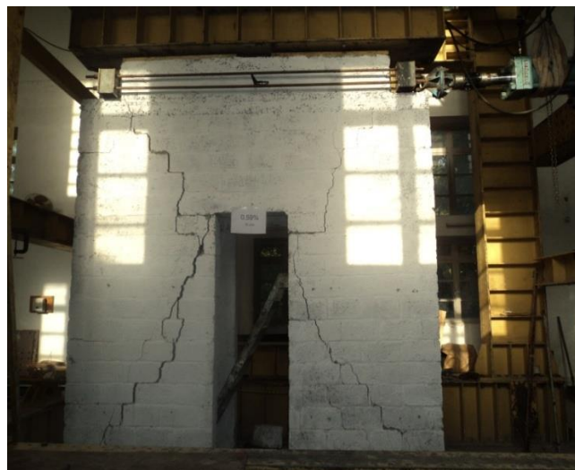
Figure 4: Diagonal Cracks Propagation in the Piers at a Story Drift of 0.26 % (8 mm displacement)
