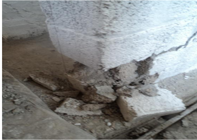
Figure 5: Crushing of Toe in Unreinforced Masonry Wall at a Story Drift of 0.53% (16 mm displacement)
