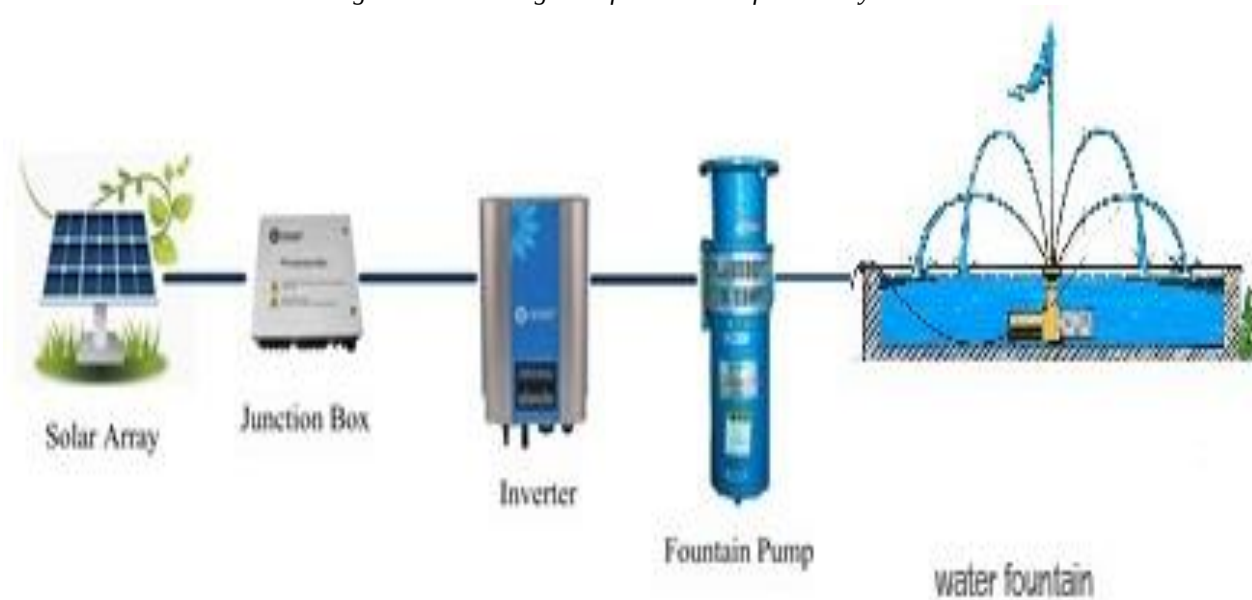
Figure 3. systematic diagram of solar PV water fountain
