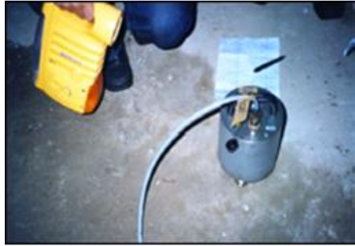
Fig 3. Ambient vibration record from the traffic load with seismometer on ground level
