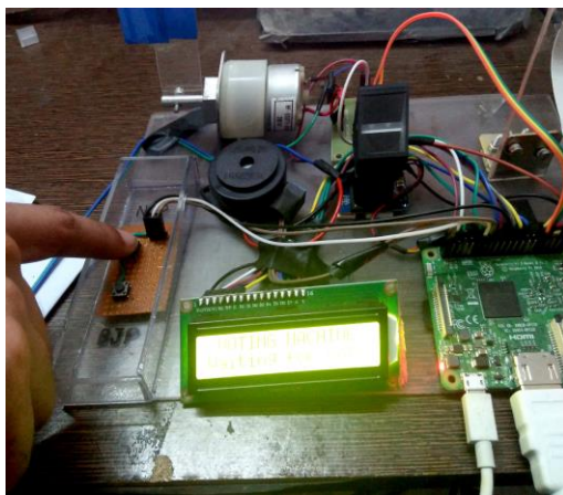
Fig 5. Voting is accepted from voter it will display result on LCD Data will be send to the cloud , so that it can be seen from any remote location.
