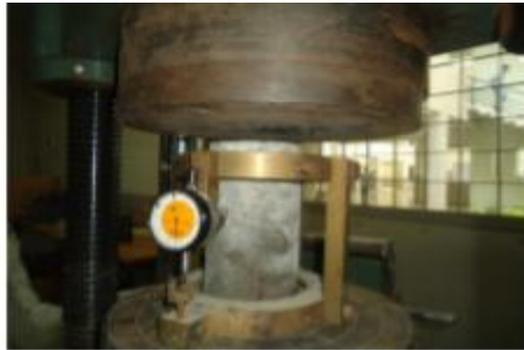
*Figure.1-Setup of Compression Test*
