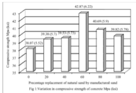
**Figure.4-Variation in compressive strength of concrete.**
