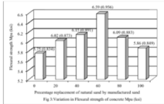
**Figure.6-Variation in Flexural strength of concrete.**
