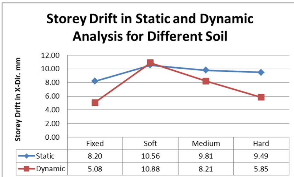
Fig. 2 Storey Drift in Static and Dynamic Analysis for Different Soil
