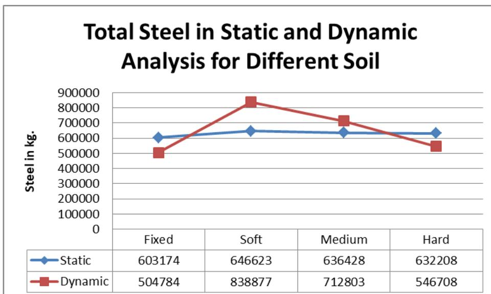
Fig. 3 Total Steel in Static and Dynamic Analysis for Different Soil
