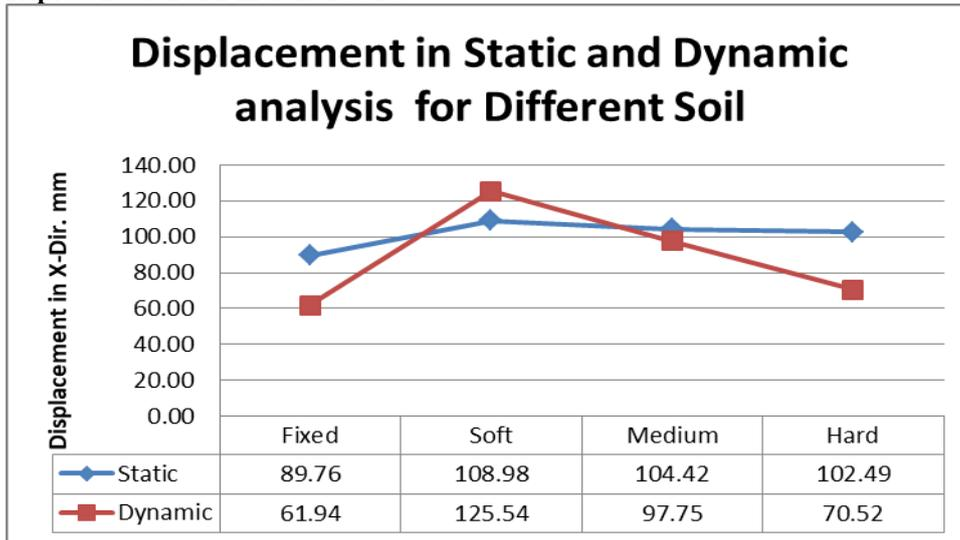
Fig. 1 Displacement in Static and Dynamic Analysis for Different Soil
