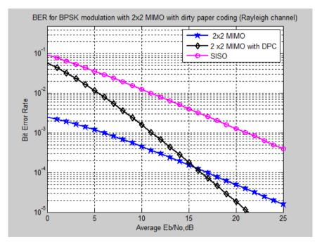
Figure 4. Bit Error Performance of SISO,2x2 MIMO and 2x2 MIMO with DPC
