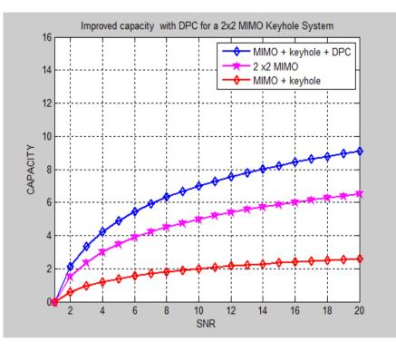
Figure 7. Improved Capacity of MIMO keyhole channel with Dirty paper coding and without DPC
