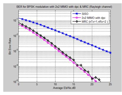
Figure 5. Bit error rate performance of 2x2 MIMO with DPC and Maximal ratio combining
