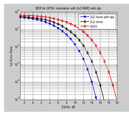
Figure 6. Improved Performance of 2x2 MIMO for QPSK using DIRTY PAPER CODING
