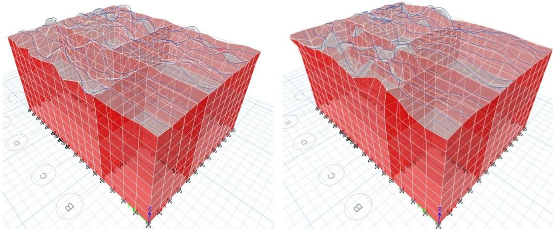
Figure 3. First mode shape (left) and second mode shape (right)
