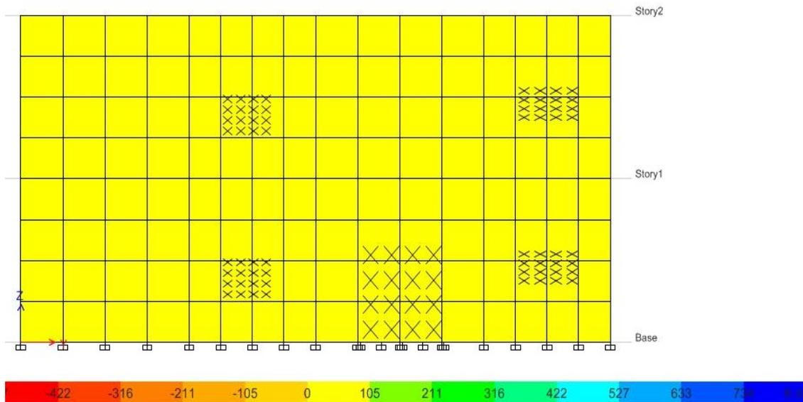
Figure 9. Maximum wall stresses for the building with CFRP (side elevation view)
