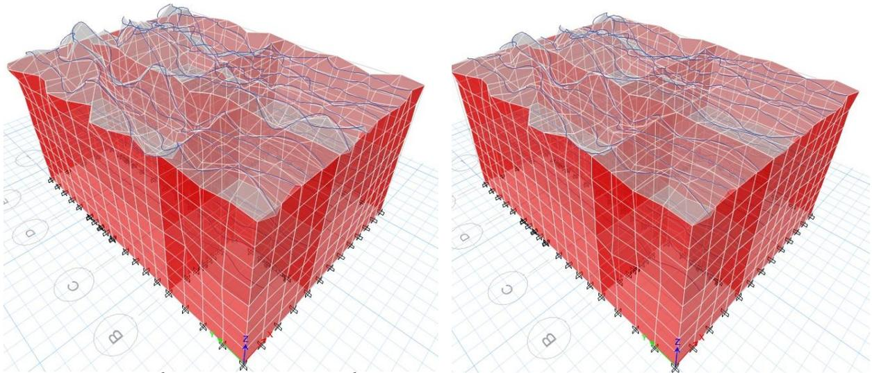
Figure 8. 3<sup>rd</sup> mode shape (left) and 4<sup>th</sup> mode shape (right) of the building strengthened by CFRP
