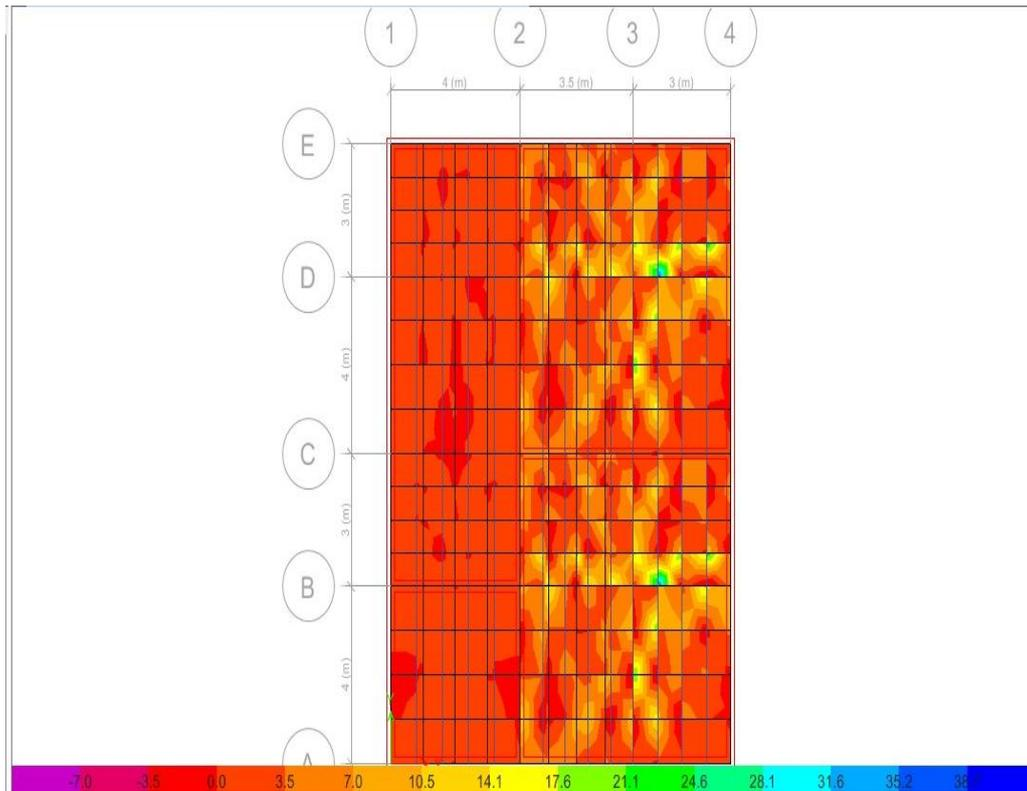
Figure 6. Maximum slab stresses of the 1st floor for building without CFRP
