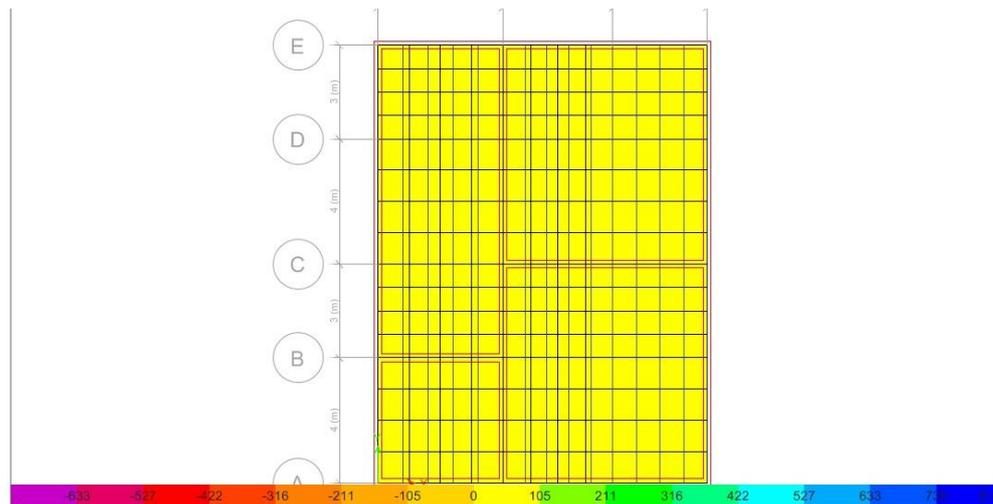
Figure.10. Maximum slab stresses of the 1st floor for building with CFRP
