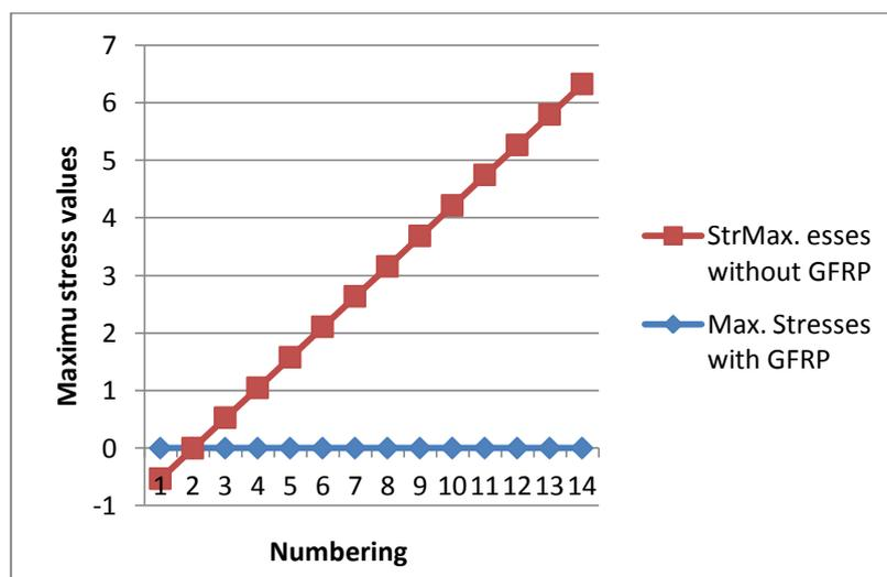
Figure 11. Comparison of stresses for building with CFRP (on walls) and without CFRP
