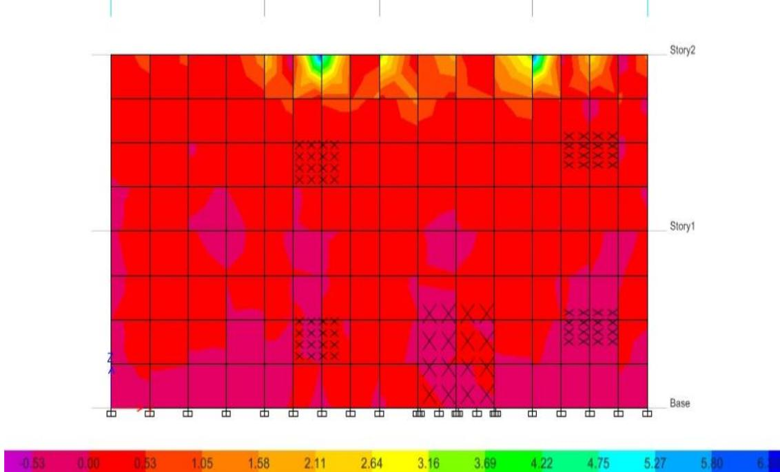
Figure 5. Maximum wall stresses for the building without CFRP (side elevation view)
