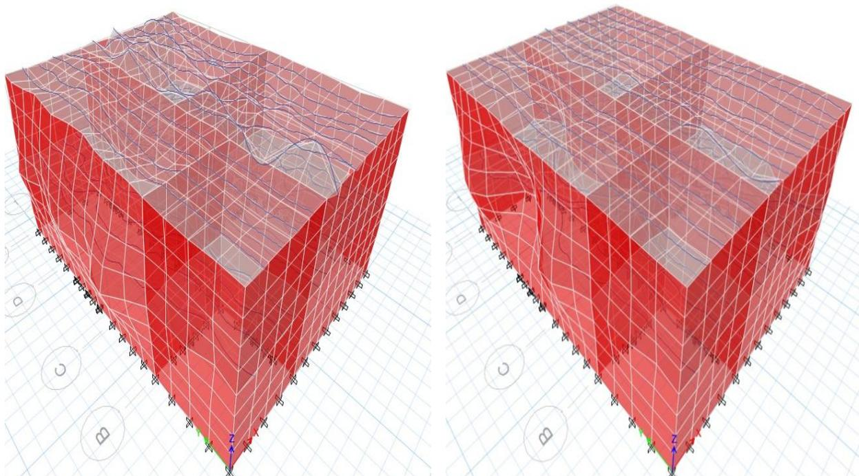
Figure 7. 1<sup>st</sup> mode shape (left) and 2<sup>nd</sup> mode shape (right) of the building strengthened by CFRP
