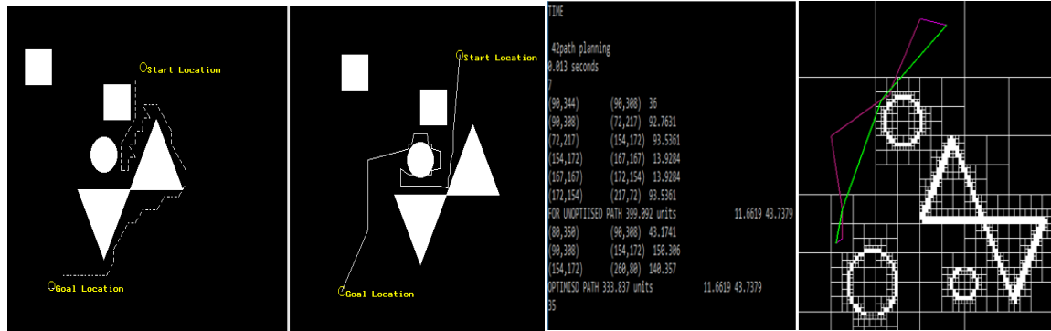
Figure 6 (a) Grid search using A* Figure (b) NFT search using Quad Figure 6 (c) D* lite
