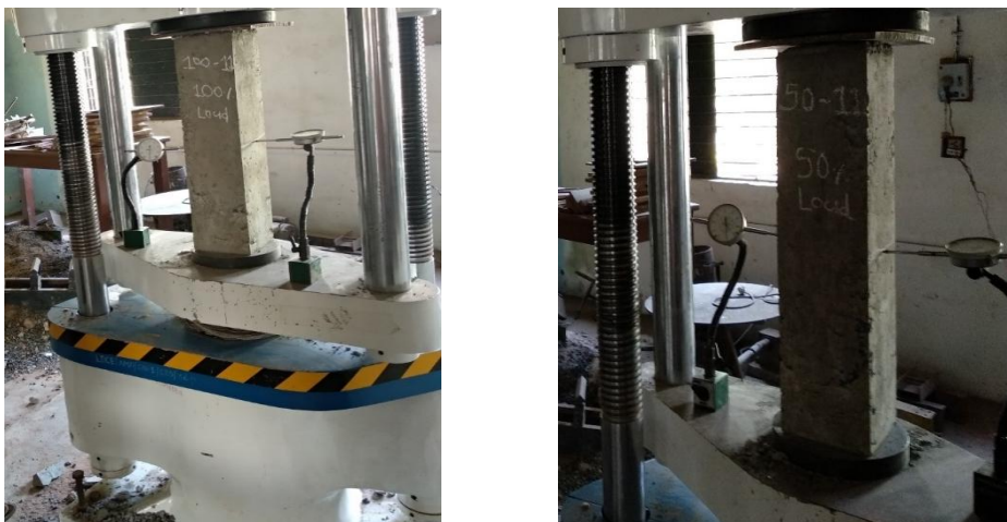
Fig.1 testing of non-jacketed column specimen
