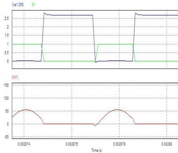
Figure-8 ZVS/ZCS turn ON and low current turn OFF of power switch
