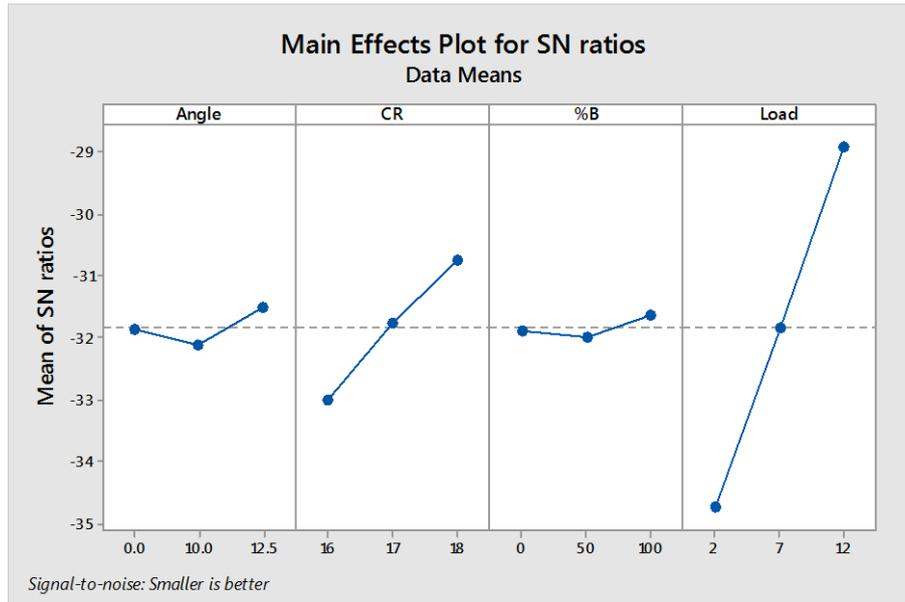
**Figure 6** Main Effects Plot for S/N ratios of HC (ppm)
