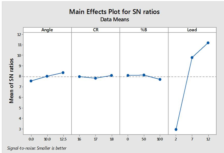
**Figure 4** Main Effects Plot for S/N ratios of Specific Fuel Consumption
