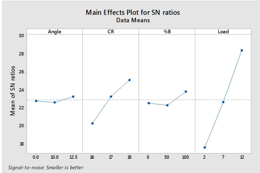
**Figure 5** Main Effects Plot for S/N ratios of CO
