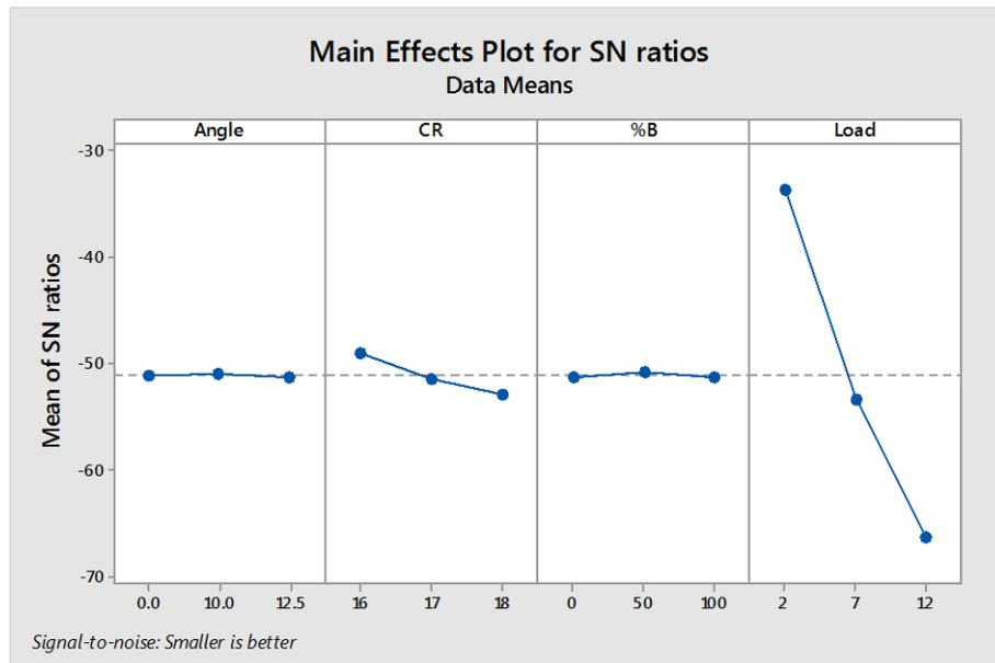
Figure 7 Main Effects Plot for S/N ratios of NO<sub>x</sub> (ppm)
