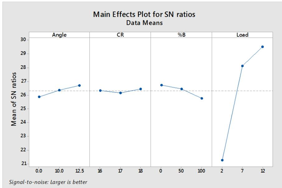
**Figure 3** Main Effects Plot for S/N ratios of Brake Thermal Efficiency
