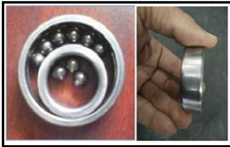
Figure 2. Ball bearing broken
