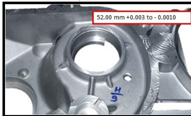
Figure 8. Housing with new tolerance
