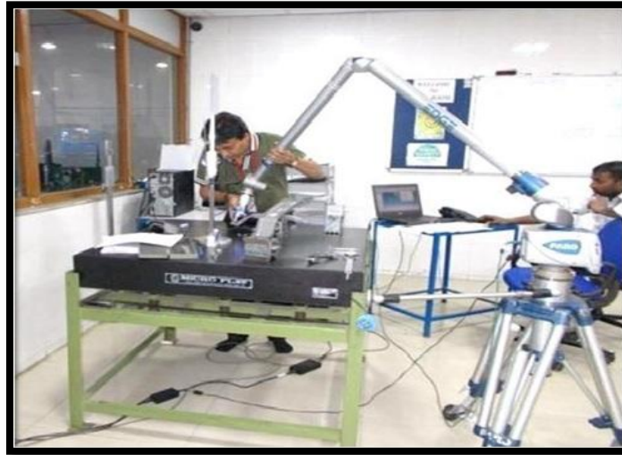
Figure 7. Measurements on CMM
