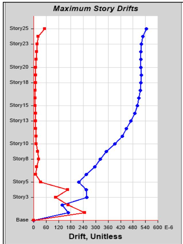
Figure 17: Story drift with damper in whole building
