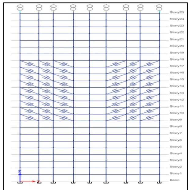
Figure 7: FVD at middle of the building (2<sup>nd</sup> case)
