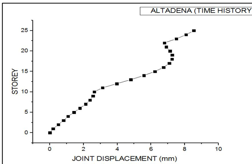
Figure 13: Displacement in X direction in Altadena case without damper
