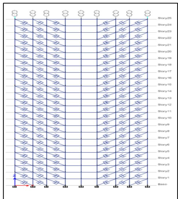
Figure 9: FVD placed in whole building (4<sup>th</sup> case)
