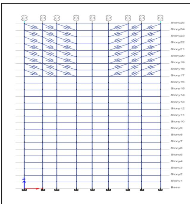
Figure 8: FVD at top of portion of building (3<sup>rd</sup> case)
