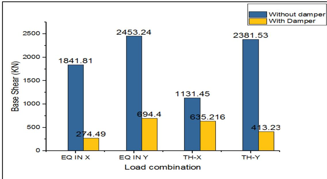
**Figure 18: Base shear Without Damper & with Damper**
