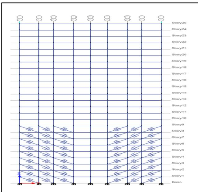
Figure 6: FVD at Bottom of the building (1<sup>st</sup> case)
