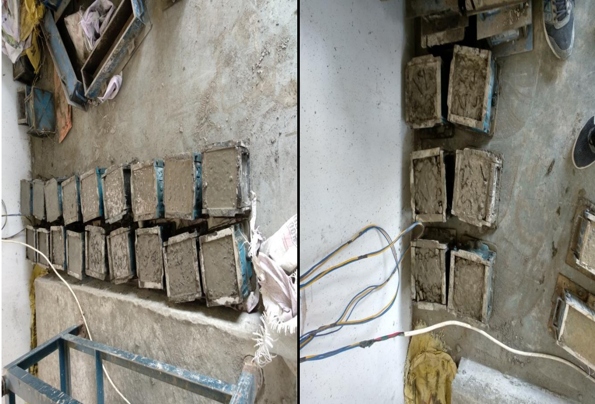
Fig 4 durability (Acid attack testing) specimens
