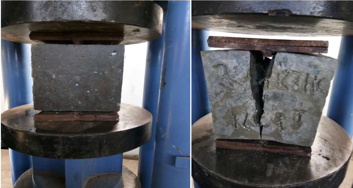
Fig 2 split tensile strength specimens
