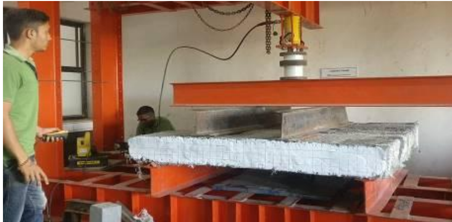
Figure 11 :- Flexure test of (MSA) Slab
