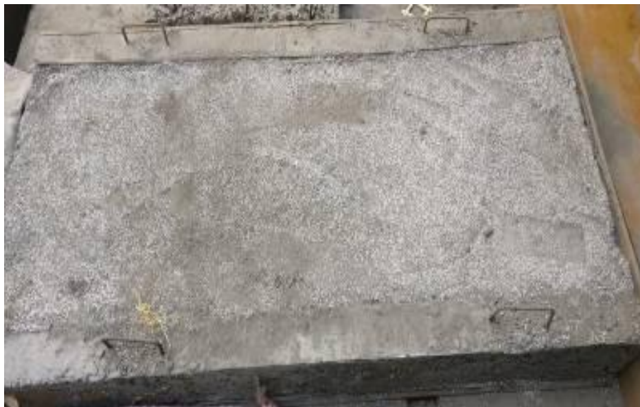
Figure 10:-Complete casting (MSB) Slab
