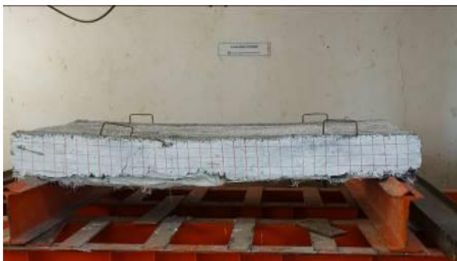
Figure 15 :- Shear Crack after test
