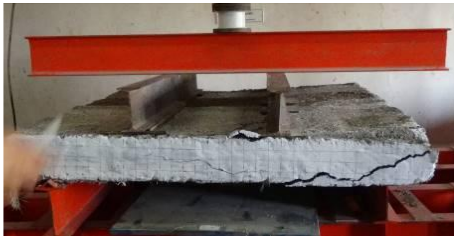
Figure 12:- Crack after test in (MSA) Slab
