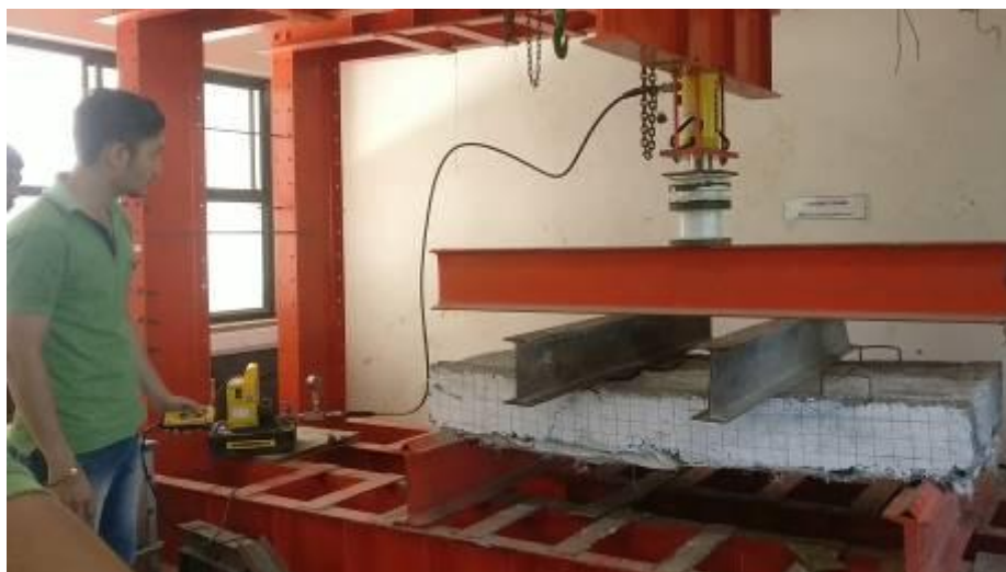
Figure 14:-Testig of the MSB Slab
