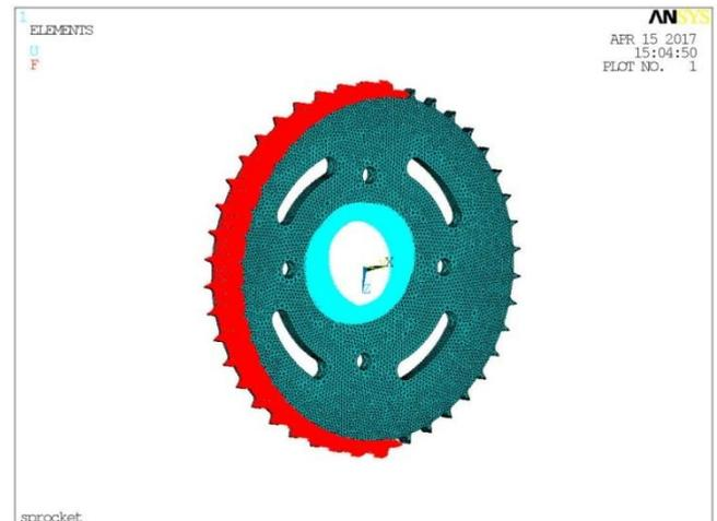
Fig.4: Meshed 3D Model with Boundary Conditions
