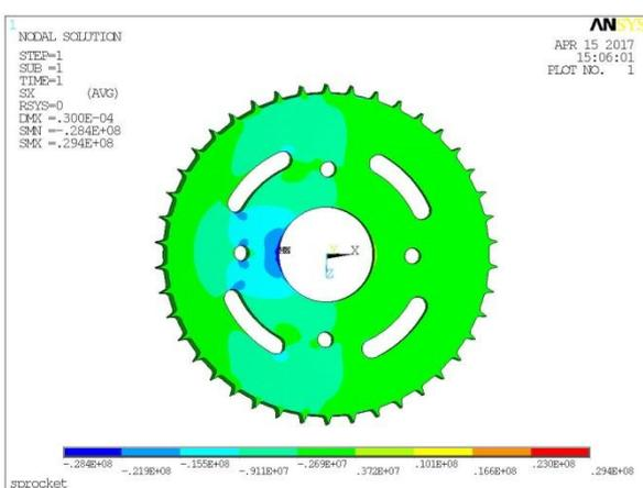
Fig.8: X component of Stress
