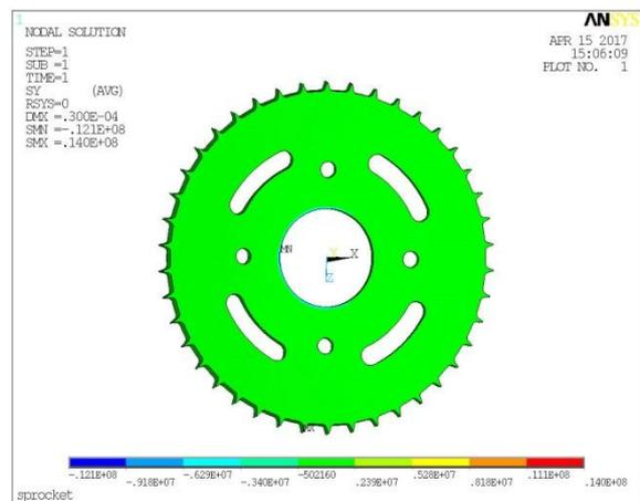
Fig.9: Y component of Stress
