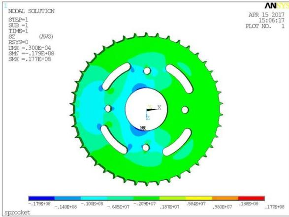
Fig.10: Z component of Stress
