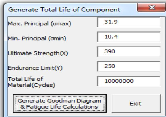
Fig.15: Input data for the Fataigue Life calculations
