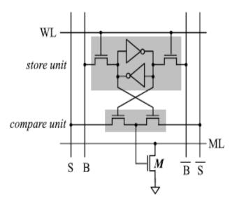
Figure 1: XOR CAM cell[1]
