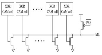
Figure 2: Conventional NOR-Type CAM[1]
