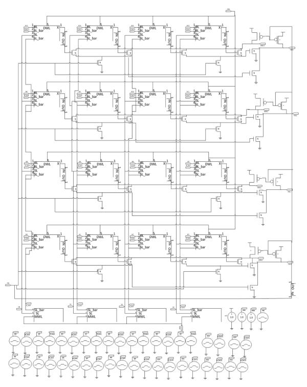
Figure 6: Schematic of 4×4 bit Modified 4T XNOR Cell MSML Design
