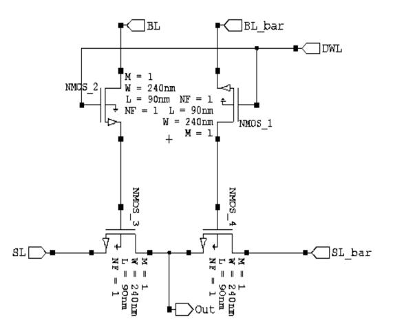
Figure 5: Modify 4T XNOR CAM Cell[2]
