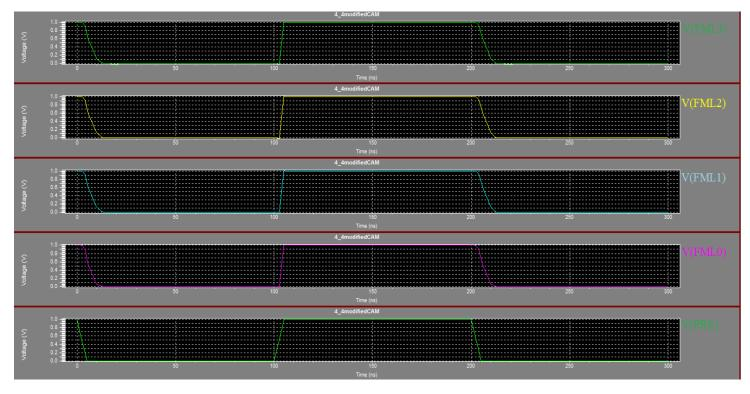
Figure 7: Transient Simulation of 4×4 bit Modified 4T XNOR CellMSML Design (Mis-match Condition)
