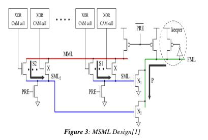
In conventional CAM, when mis-match condition occurred at that time MML discharged to 0. In MSML design, charge loss is less because only mis-match SMLs charges from MML and then discharge before dis-charging the overall MML to 0.After MML, SML and FML(Final Matching-Line) use to define match- result.
