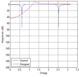
Figure 12. Magnitude response of chebyshev type 2 band pass filter (attempt\_max=5)
