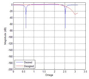
Figure 9. Magnitude response of chebyshev type 2 band pass filter (attempt\_max=1)
