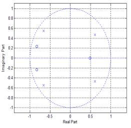
Figure 7. Pole-zero plot of butterworth band pass filter (attempt\_max=5)
