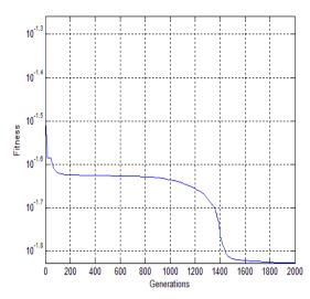
Figure 11. Fitness curve of chebyshev type 2 band pass filter (attempt\_max=1)
