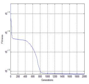
Figure 14. Fitness curve of chebyshev type 2 band pass filter (attempt\_max=5)
