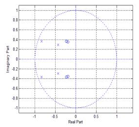
Figure 4. Pole-zero plot of butterworth band pass filter (attempt\_max=1)
