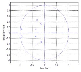
Figure 10. Pole-zero plot of chebyshev type 2 band pass filter (attempt\_max=1)
