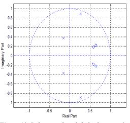
Figure 13. Pole-zero plot of chebyshev type 2 band pass filter (attempt\_max=5)
